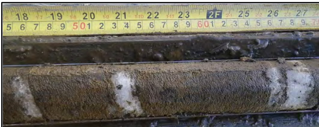
Figure A-14. Quasi-syngenetically frozen silt (intermediate layer), with micro-braided to microatactic cryostructure and thick ice belts (Sub-unit 2B), T3-107, depth 90 cm to 110 cm (35 in. to 43 in.).
