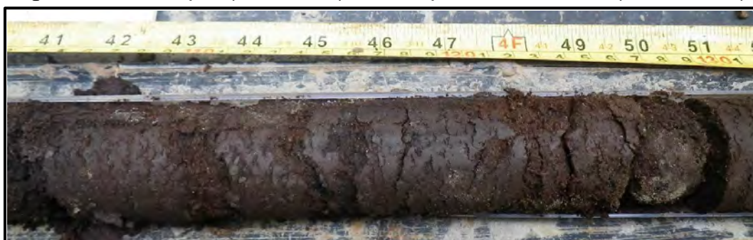
Figure A-1. Unfrozen peat (Sub-unit 2UF), T3-50, depth 110 cm to 140 cm (43 in. to 55 in.).
