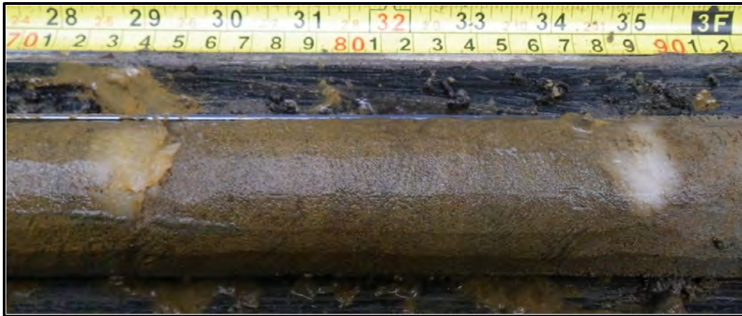
Figure A-6. Ice-rich syngenetically frozen silty sand, very fine to fine, strongly oxidized, with micro-braided cryostructure and thick ice belts (Sub-unit 6A), T3-62, depth 210 cm to 230 cm (83 in. to 90 in.).
