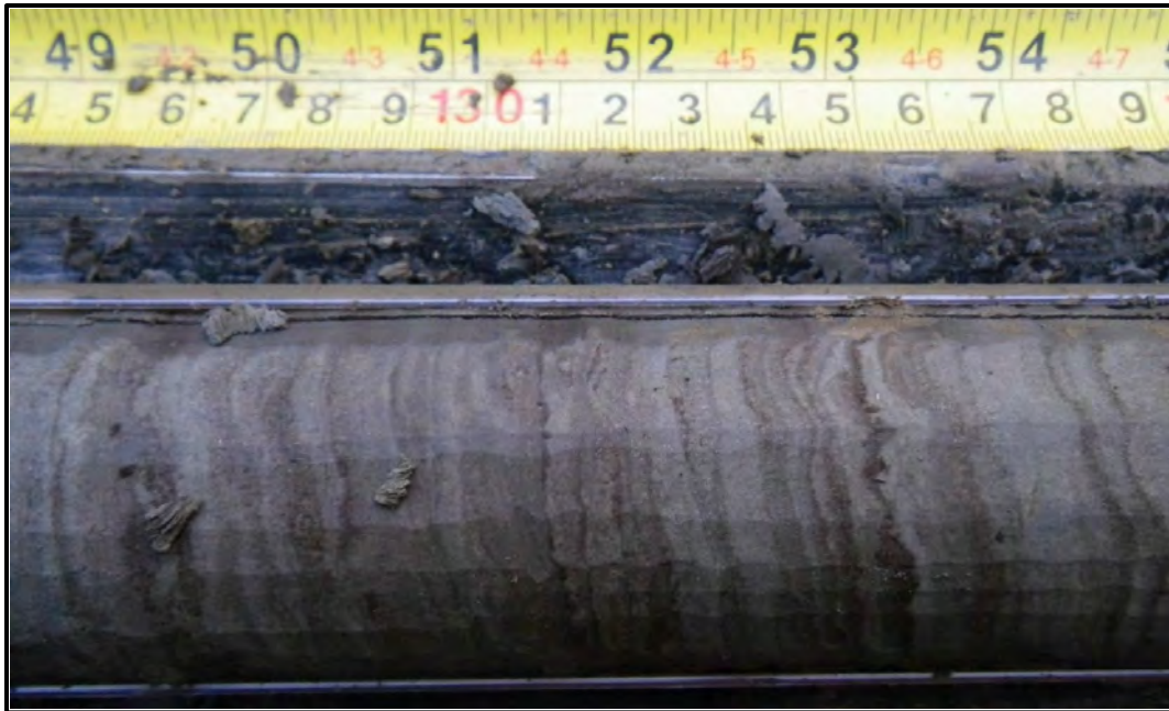
Figure A-17. Epigenetically frozen laminated silty sand / very fine to fine sandy silt with thin layers of organic detritus (Sub-unit 6B), no visible ice, T3-137, depth 370 cm to 380 cm (145 in. to 149 in.).
