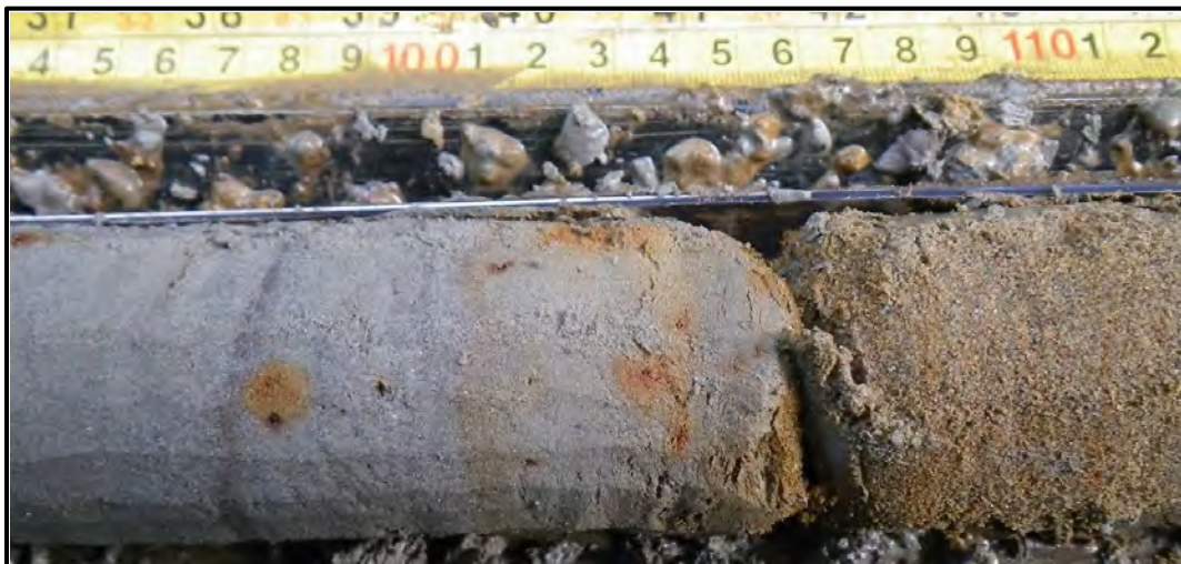
Figure A-4. Boundary between ice-poor epigenetically frozen sandy silt (Sub-unit 6B) and ice-poor epigenetically frozen fine to medium sand (Unit 7), T3-56, depth 380 cm (149 in.).
