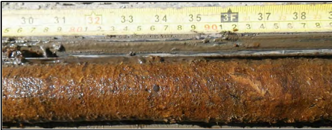
Figure A-15. Quasi-syngenetically frozen peat (buried), with organic-matrix to microatactic cryostructure (Sub-unit 4B), T3-107, depth 220 cm to 240 cm (86 in. to 94 in.).
