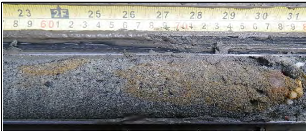
Figure A-12. Boundary between epigenetically frozen sand, fine to medium, with inclusions of very coarse sand (Unit 7) and sandy gravel (Sub-unit 8B), no visible ice, T3-98, depth 670 cm (263 in.).
