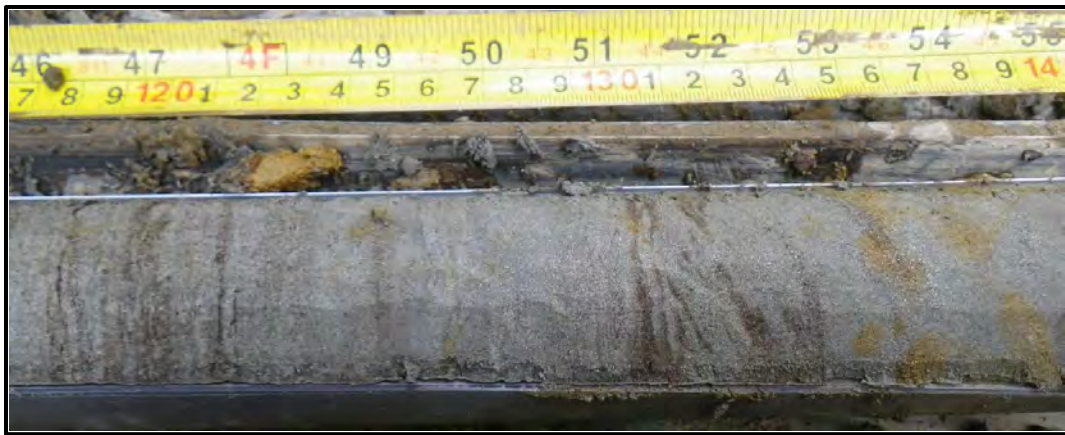
Figure A-9. Epigenetically frozen very fine to fine silty sand, with thin layers of organic detritus (Sub-unit 6B), no visible ice, T3-68, depth 390 cm to 410 cm (153 in. to 161 in.).
