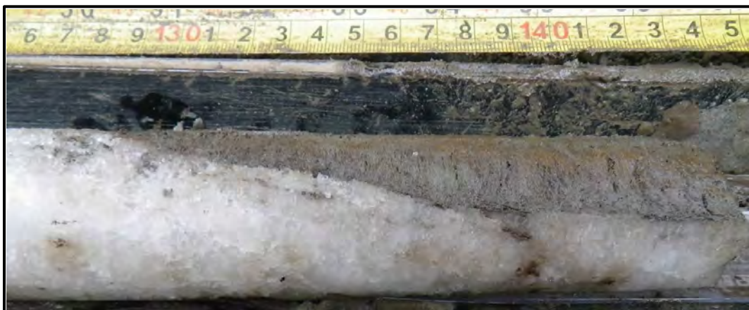
Figure A-5. Contact between the ice wedge and the ice-rich syngenetically frozen silt with micro-braided cryostructure (Sub-unit 3A), T3-62, depth 135 cm to 150 cm (53 in. to 59 in.).
