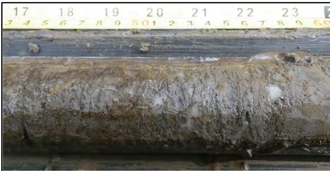
Figure A-10. Ice-rich quasi-syngenetically frozen silt with ataxitic cryostructure (Sub-unit 3A), T3-71, depth 185 cm to 200 cm (73 in. to 79 in.).
