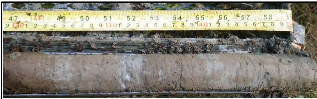
Figure A-3. Thawed and refrozen organic-rich silt with lenticular to layered cryostructure (Sub-unit 3B), T3-56, depth 120 cm to 150 cm (47 in. to 59 in.).
