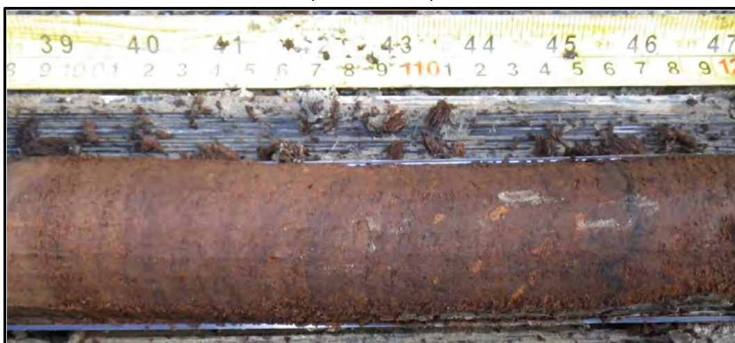
Figure A-2. Frozen peat, no visible ice (Sub-unit 2A), T3-56, depth 90 cm to 110 cm (35 in. to 43 in.).
