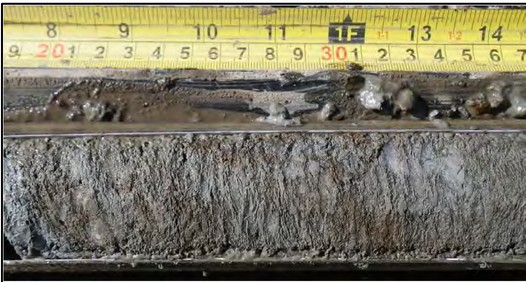
Figure A-16. Quasi-syngenetically frozen silt (buried intermediate layer), with braided to atactic cryostructure (Sub-unit 5A), T3-107, depth 280 cm to 295 cm (110 in. to 116 in.).
