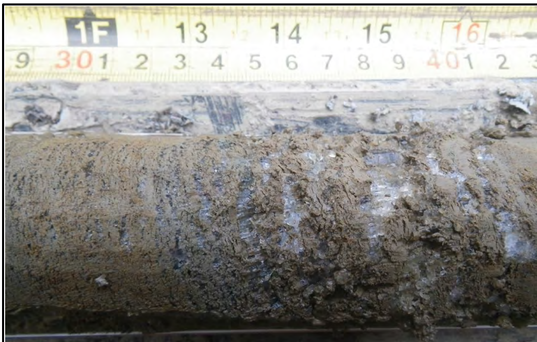
Figure A-18. Quasi-syngenetically frozen silt (intermediate layer), with braided to ataxitic cryostructure (Sub-unit 3A), T3-146, depth 70 cm to 80 cm (28 in. to 31 in.).
