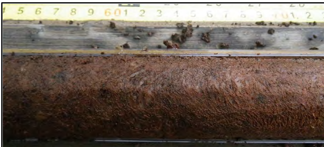
Figure A-8. Ice-rich quasi-syngenetically (or syngenetically) frozen peat with organic-matrix to micro-braided and ataxitic cryostructure and thick ice belts (Sub-unit 2B), T3-68, depth 80 cm to 95 cm (31 in. to 37 in.).
