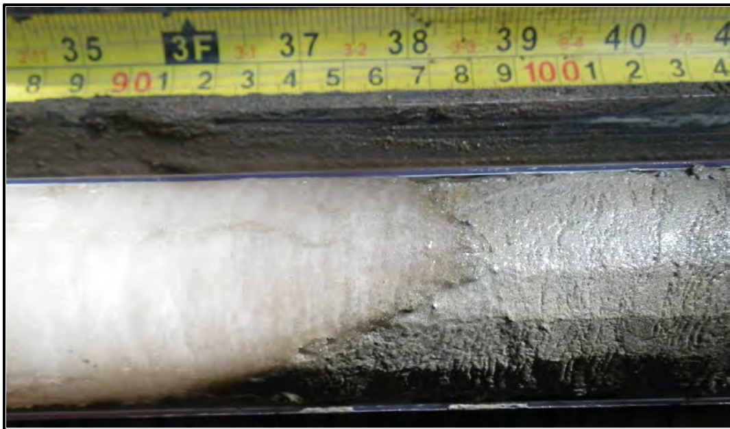
Figure A-11. Contact between the ice wedge and syngenetically frozen sandy silt with micro-layered cryostructure (Sub-unit 6A), T3-83, depth 225 cm to 235 cm (88 in. to 92 in.).
