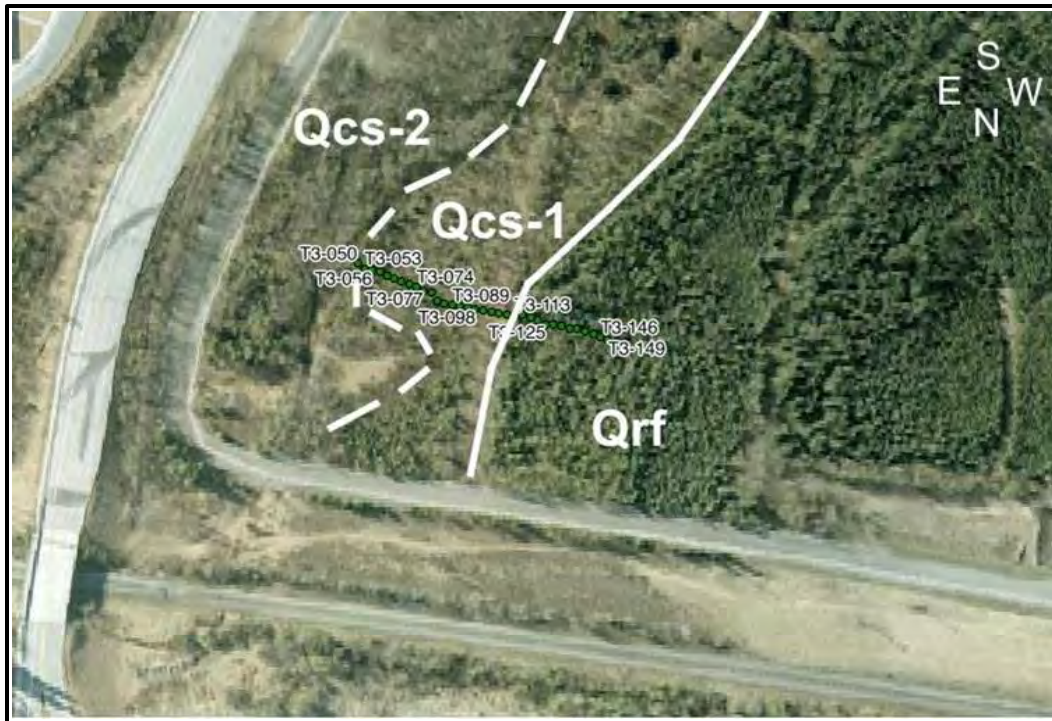
Figure 30. Surface terrain features map for the CCHRC test location showing borehole sample locations and transition boundaries between terrain units. Terrain units (geology) are Qrf, Alluvial-Fan Silt (overlies floodplain alluvium); perennially frozen; Qcs, Swale and slough deposits (silt and silty sand, contains organic material); Qcs-1, perennially frozen near the surface; and Qcs-2, lowered permafrost table (after Péwé et al. 1977). Map orientation, south up, correspond to data analysis in Fig. 31.
