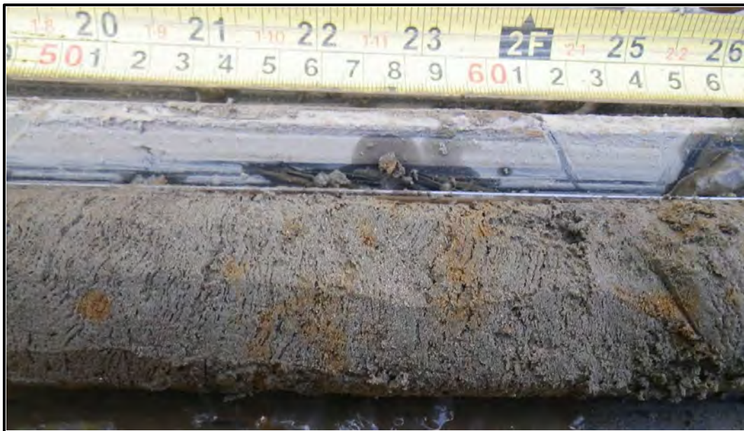
Figure A-13. Syngenetically frozen silty sand, friable, with micro-layered cryostructure (Sub-unit 6A), T3-101, depth 310 cm to 315 cm (122 in. to 124 in.).
