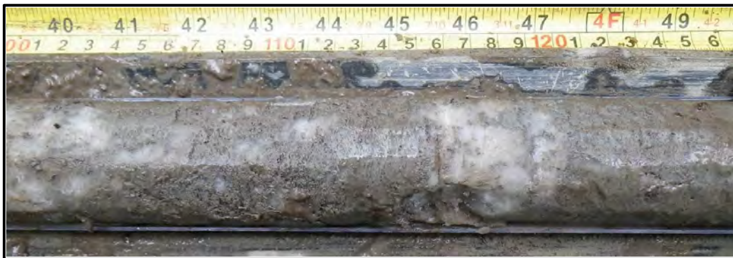
Figure A-7. Ice-rich quasi-syngenetically frozen silt (intermediate layer) with ataxitic cryostructure and thick ice belts (Sub-unit 3A), T3-65, depth 110 cm to 130 cm (43 in. to 51 in.).
