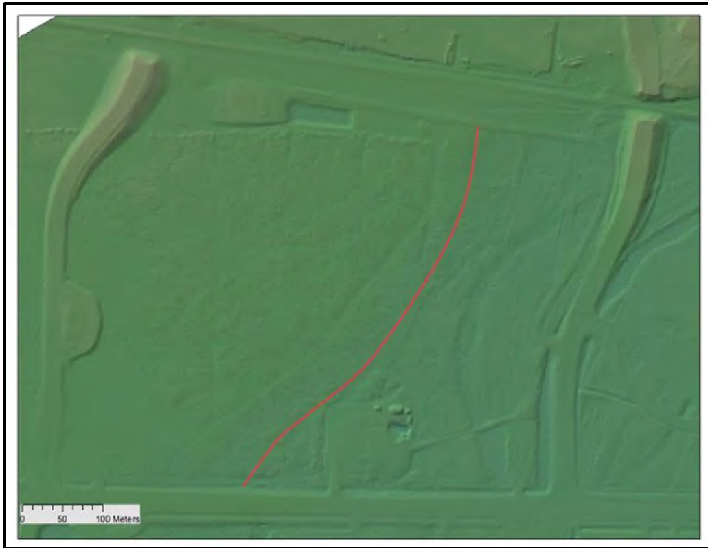
Figure 4. Recent false color LiDAR image of the CCHRC test site in 2010, with elevational changes shown. Patterns indicative of former stream channels or sloughs are evident in the eastern third of the image to right of the red line. Alluvial-fan deposits lie to the left of the red line. Trails through vegetation occur in the western two-thirds; roads with embankments are clearly evident.
