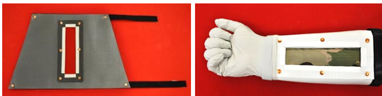
Figure 10. Left: Sleeve device used for arm-in-cage bioassays; Right: arm-in-cage sleeve attached to study participant.
