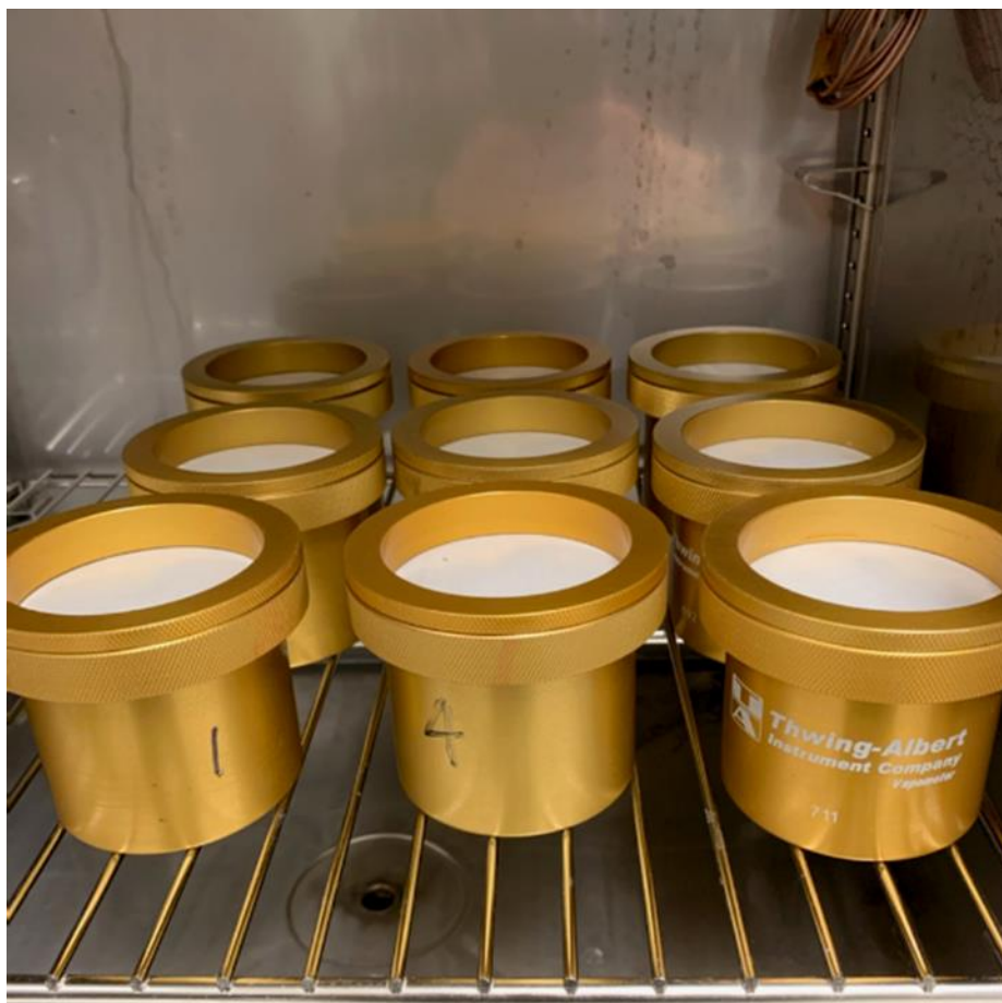
Figure 14. Holders utilized for WVTR test inside Luna's environmental chamber.
