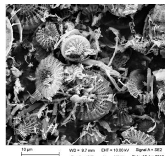
Figure 2. SEM of diatomaceous earth material
