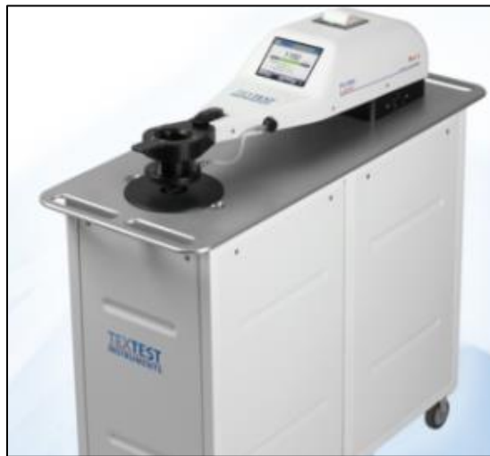
Figure 13. Representative Testex FX 3300 used at Clemson University for ASTM D737 air permeability testing.
