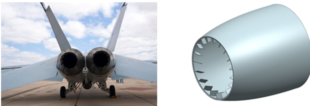
Figure 1. Schematic of swirl vanes near the nozzle exit(s) for noise reduction (not-to-scale)
