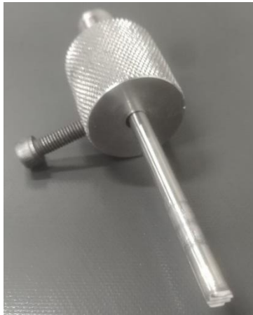
Figure 15.2. Photograph of the deglazing punch developed for the disruption of the material within the column to deglaze and relieve material stresses located at the press interfaces.
