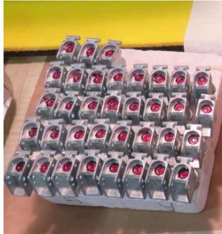
Figure 10.2. Photograph of M201A1 fuze assemblies after varnishing with the required lacquer.
