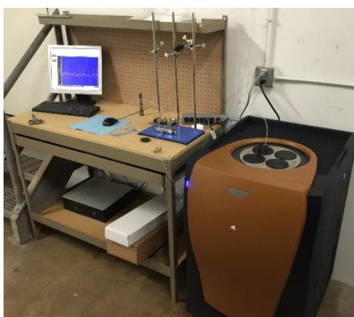
Figure 5.1. Photograph of TAM IV Microcalorimeter located at IMP.
