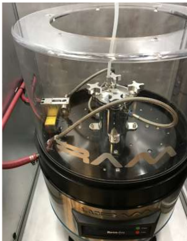
Photograph 7.2.5-1: Vessel with Cooling Jacket Secured to Mixer
