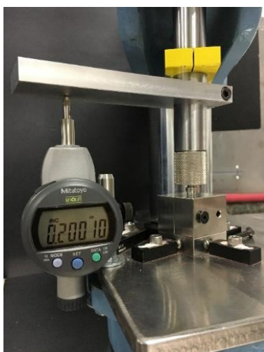
Figure 6.10. Photograph of IMP developed delay column material consolidation height measurement system.
