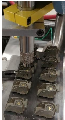
Figure 15.5. Inserting primed primer assemblies into fuze bodies during manufacturing process.
