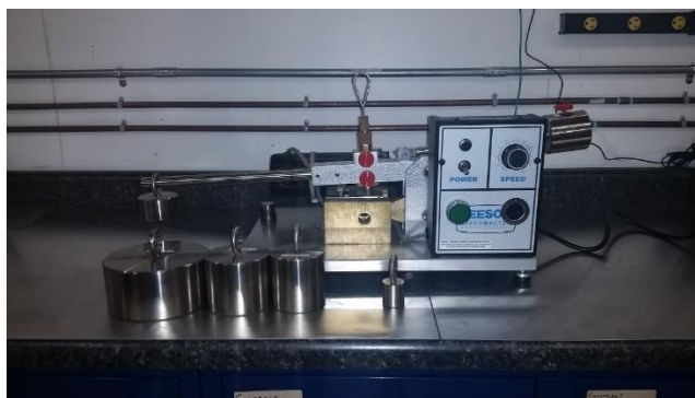
Figure 14.2. Photograph showing BAM friction sensitivity tester at Innovate Materials and Processes, LLC (Purchased from Chilworth Technology Ltd.).
