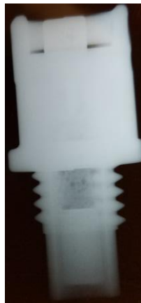
Figure 10.3. Photograph of M201A1 fuze assembly x-ray.
