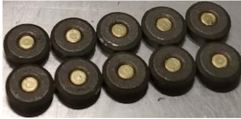
Figure 15.4. Photograph of M42 primers inserted into M213A1/M228A1 primer holders.
