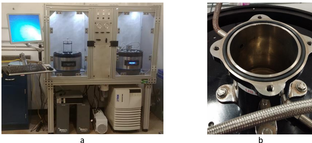
Figure 7.4. (a) Resodyn LabRAM mixers with integrated cooling and vacuum systems. (b) Jacketed mixing vessel used for mixing of the environmentally benign delay formulation.
