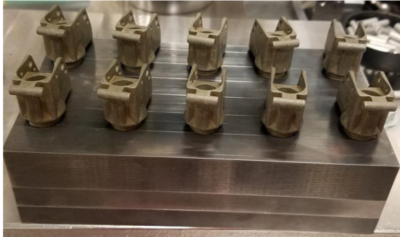
Figure 15.1. Photograph of M213/M228 fuzes in the consolidation die.
