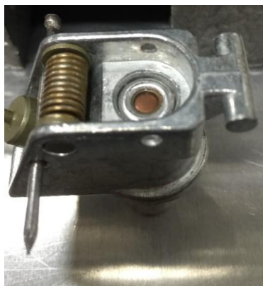
Figure 8.1. Photograph of M201A1 environmentally benign delay column with M39A1C primer crimped and inserted in the grenade delay column housing.
