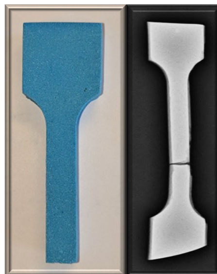
Figure 7. Typical cured PBXN-110 surrogate dog bone (left) and X-ray image of the same (right).
