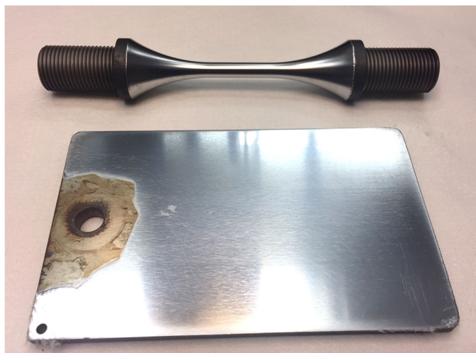
Figure 21. Photograph of exemplary Cr-plated 4340 steel dogbone tensile specimens and 4340 steel corrosion test panels obtained from CCAD.
