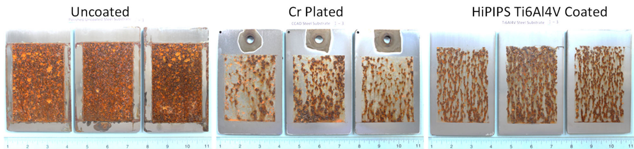
Figure 22. Photographs of samples after 15 cycles of GMW 14872 testing on 4340 steel substrates. The coatings tested included the SwRI-developed HiPIPS coatings as well as coatings applied using conventional plating techniques and uncoated samples for comparison.
