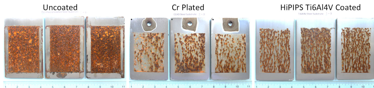
Figure E-7. Photographs of samples after 15 cycles of GMW 14872 testing on 4340 steel substrates.
