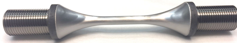
Figure 6. Schematic and photograph of S-N dogbone specimens for mechanical testing.
