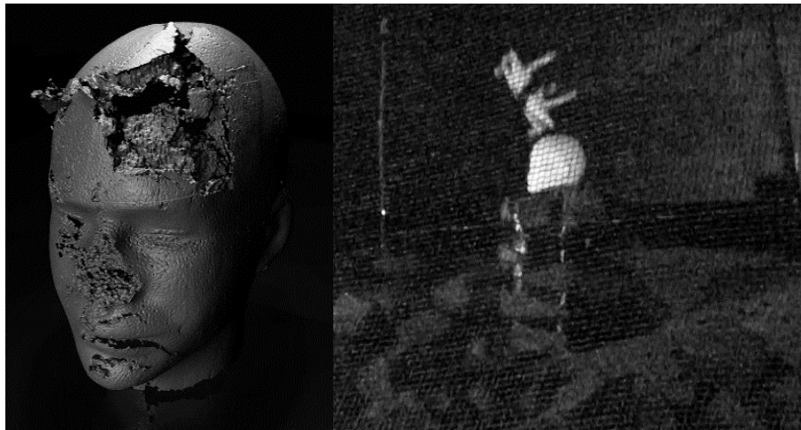
(a) Styrofoam head showing impact damage from rotated quadcopter.
