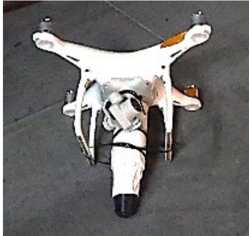
FIGURE 9. Phantom 4 Pro With Custom Payload—Improved Explosive Device (IED) Surrogate.
