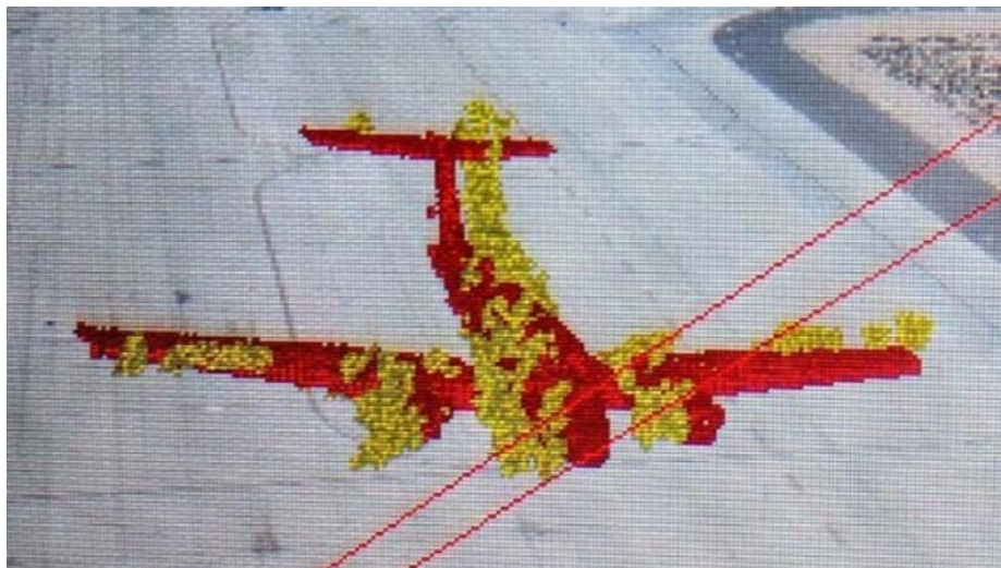
Figure 1. C-12 Reference Model and Point Cloud.
