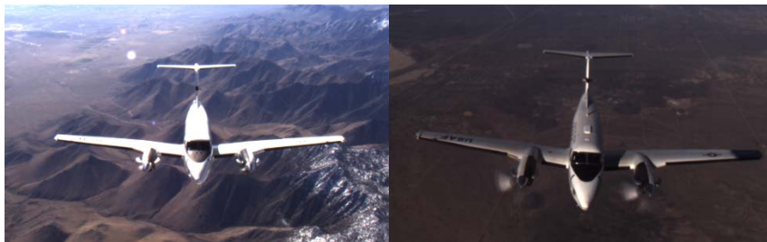
Figure 9: Camera Exposure Setting Differences from 15,000 \mu s to 5,000 \mu s
