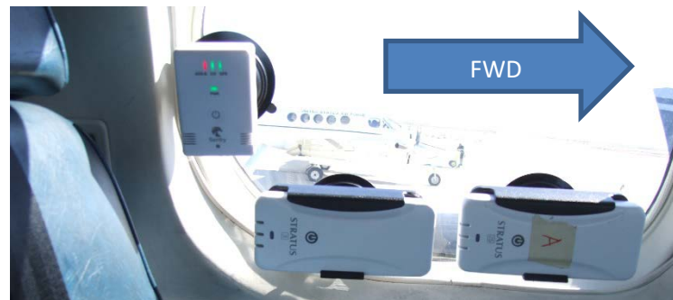
Figure 8: C-12 AHRS Capable SUT Installation
