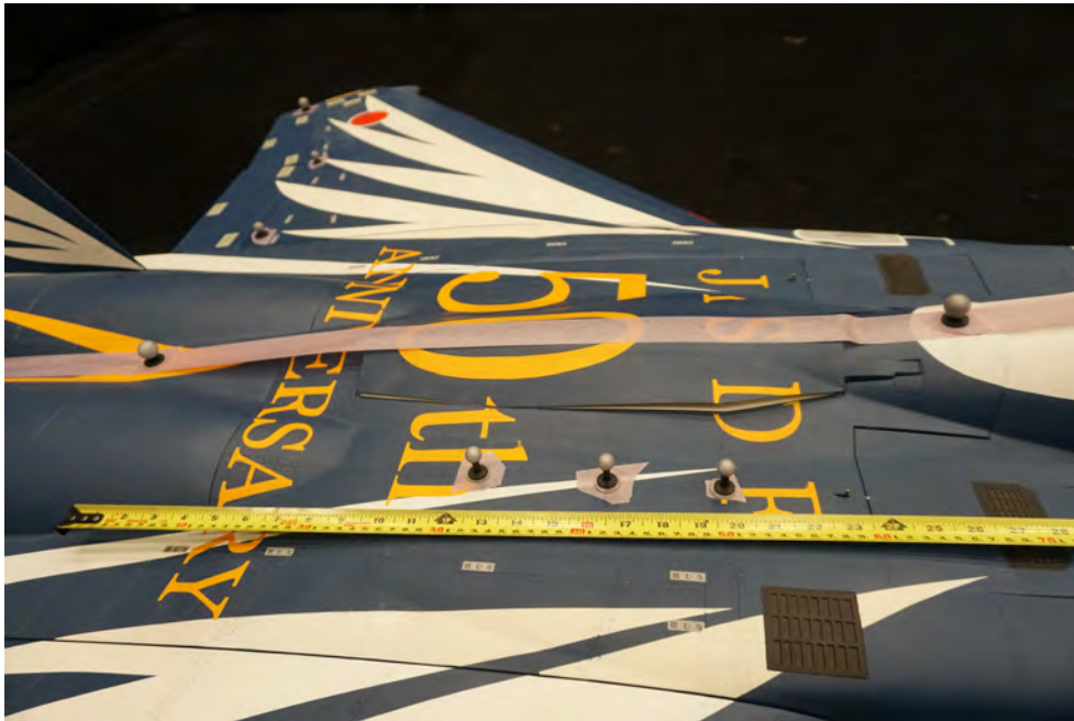
Figure 26: Reference image of the F-15's fuselage with a measuring tape for scale. Note that the center panel with the "0" is not aligned properly.
