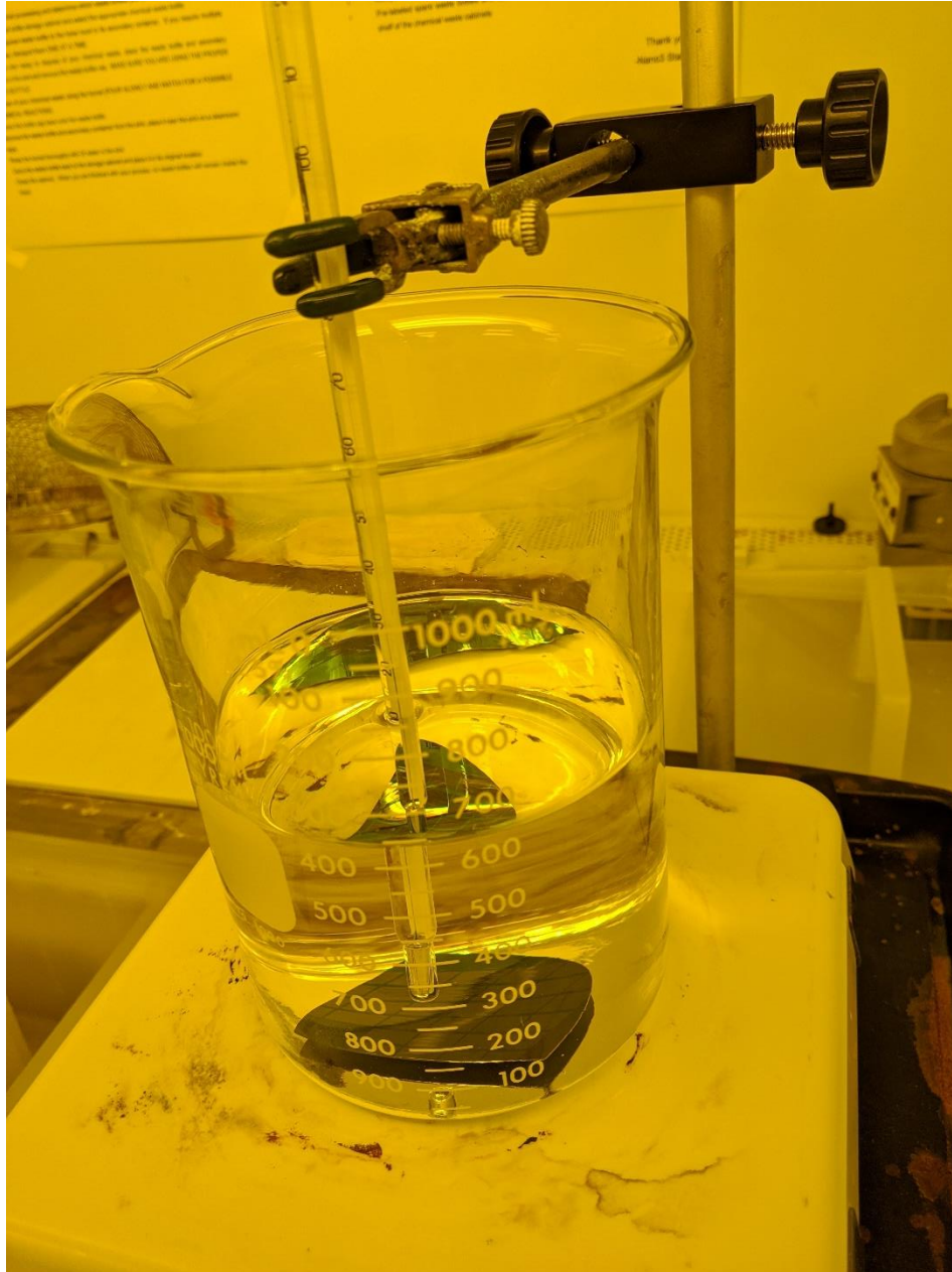
Figure 32. Image of the hot phosphoric acid etching step in the fabrication process. A beaker is filled with 600 mL of phosphoric ( \text{H}_3\text{PO}_4 ) acid and is placed on a hot plate.
