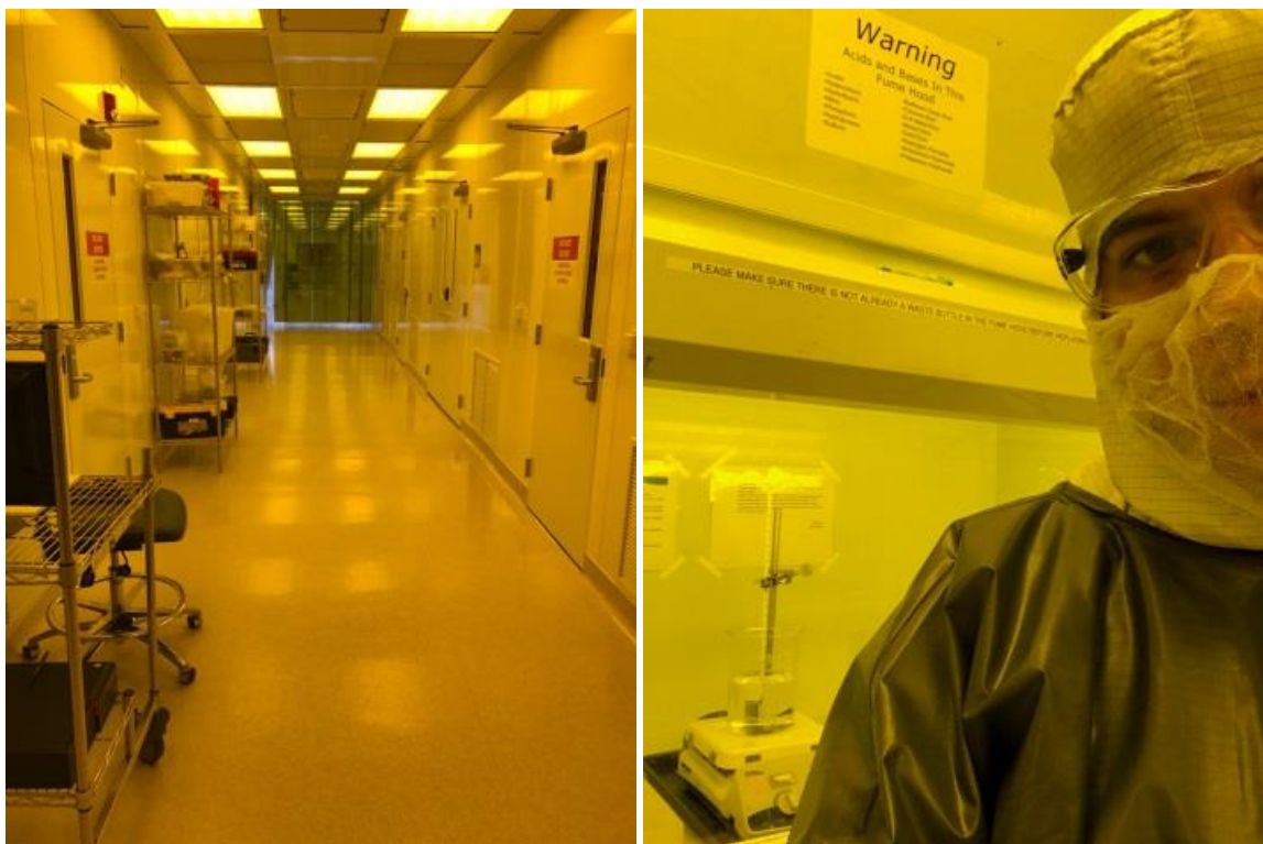
Figure 13. (Left) The main corridor of the UCSD Nano3 cleanroom facility. (Right) The PI (Dr. Torres) performing a heated phosphoric acid etching of silicon nitride ( \text{Si}_3\text{N}_4 ) in the cleanroom.
