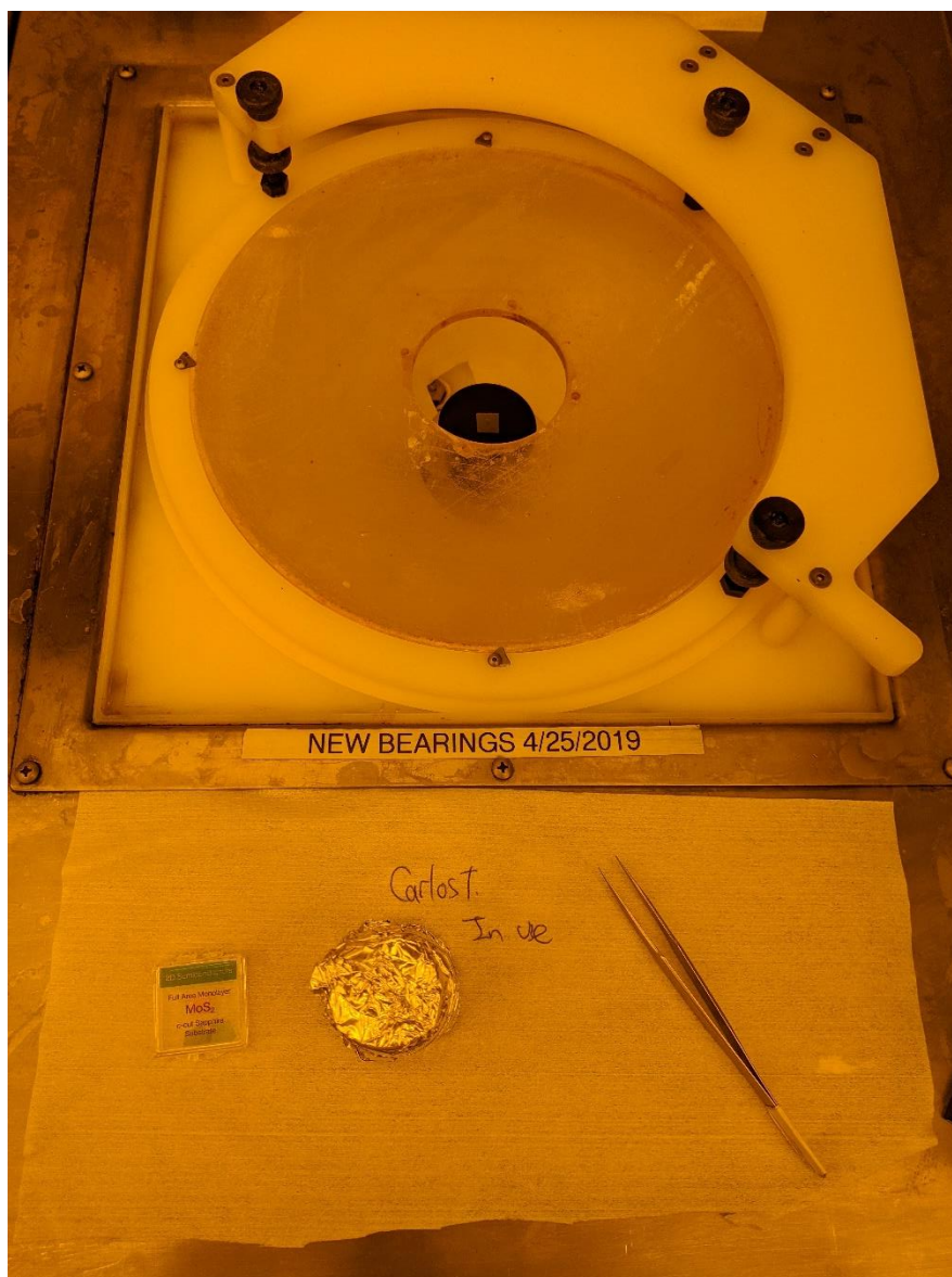
Figure 43. Spin coating PMMA polymer onto the CVD 2D material on top of sapphire substrate to assist the 2D material wet transfer onto arbitrary substrates.
