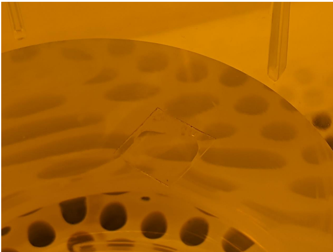
Figure 47. Close up view of the CVD 2D material/sapphire substrate floating on the surface of the BOE solution in the beaker shown in Figure 46.
