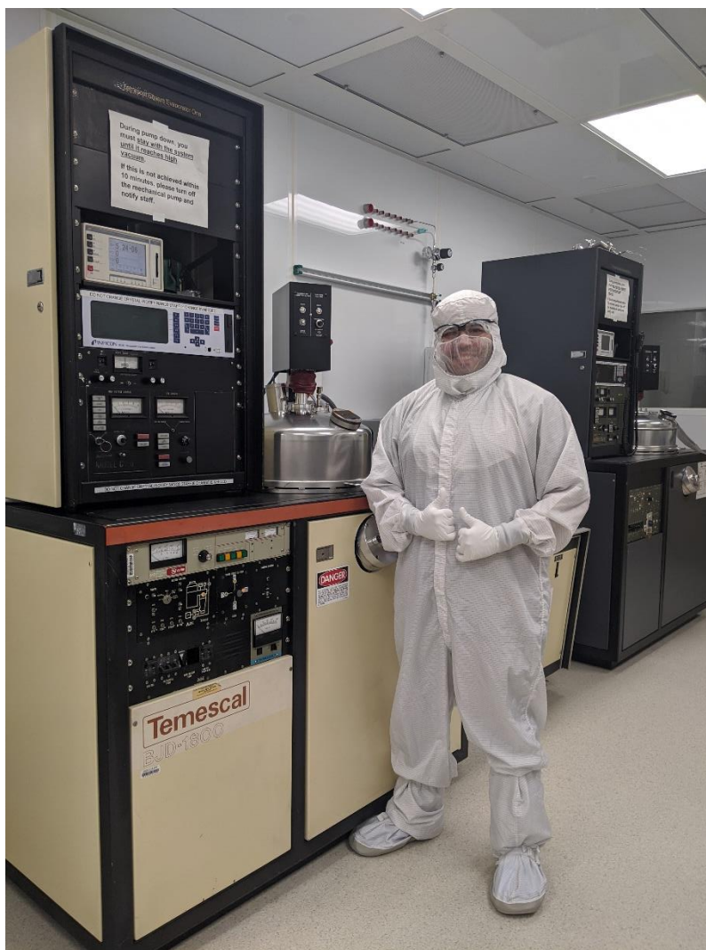
Figure 53. The PI performs metallization on the 2D-LET substrates using a Temescal BJD 1800 e-beam evaporator in the UCSD Nano3 cleanroom.
