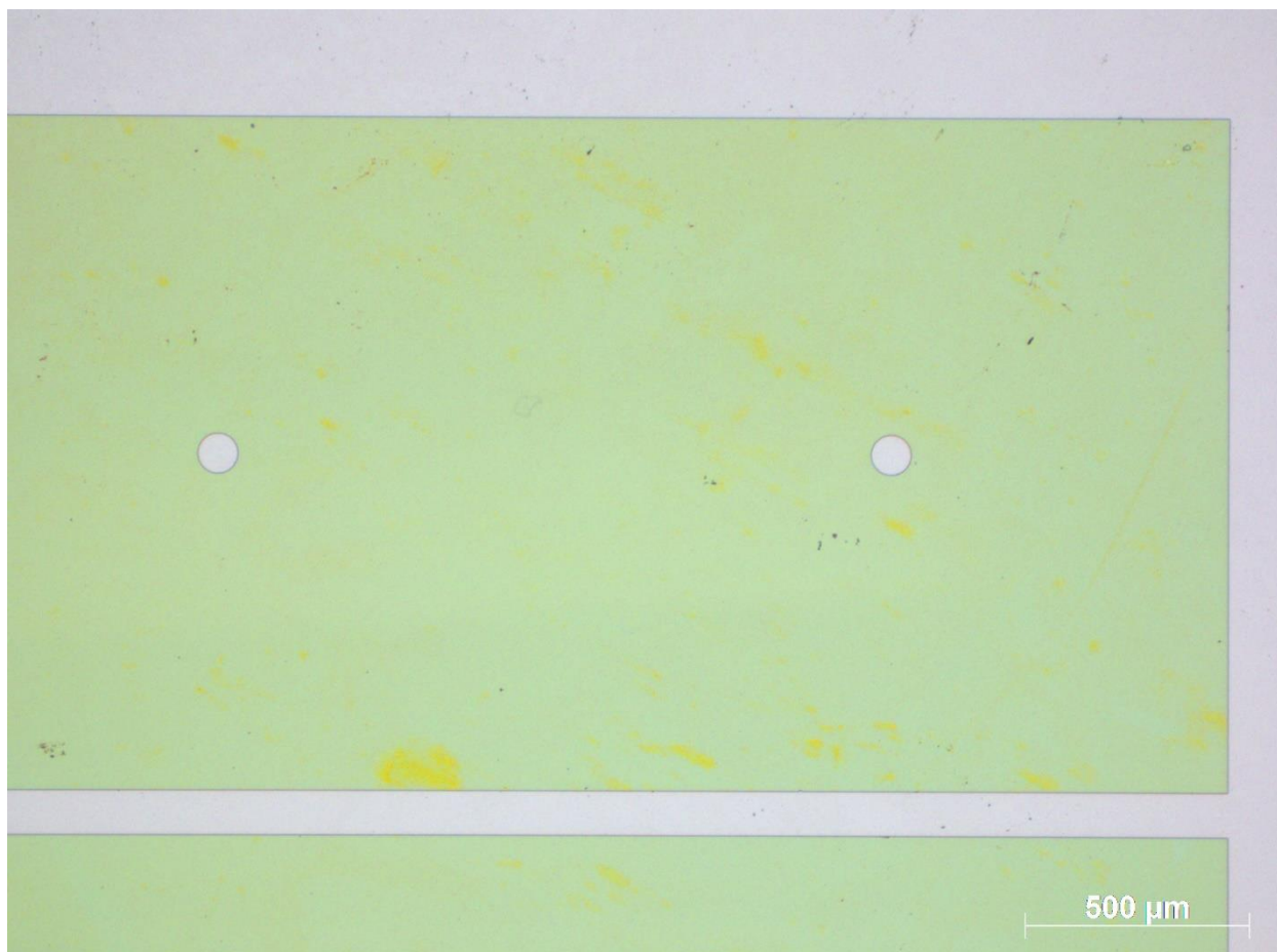
Figure 52. Optical micrograph of a 2D-LET substrate after the PMMA on top of the CVD 2D material was dissolved in acetone overnight.
