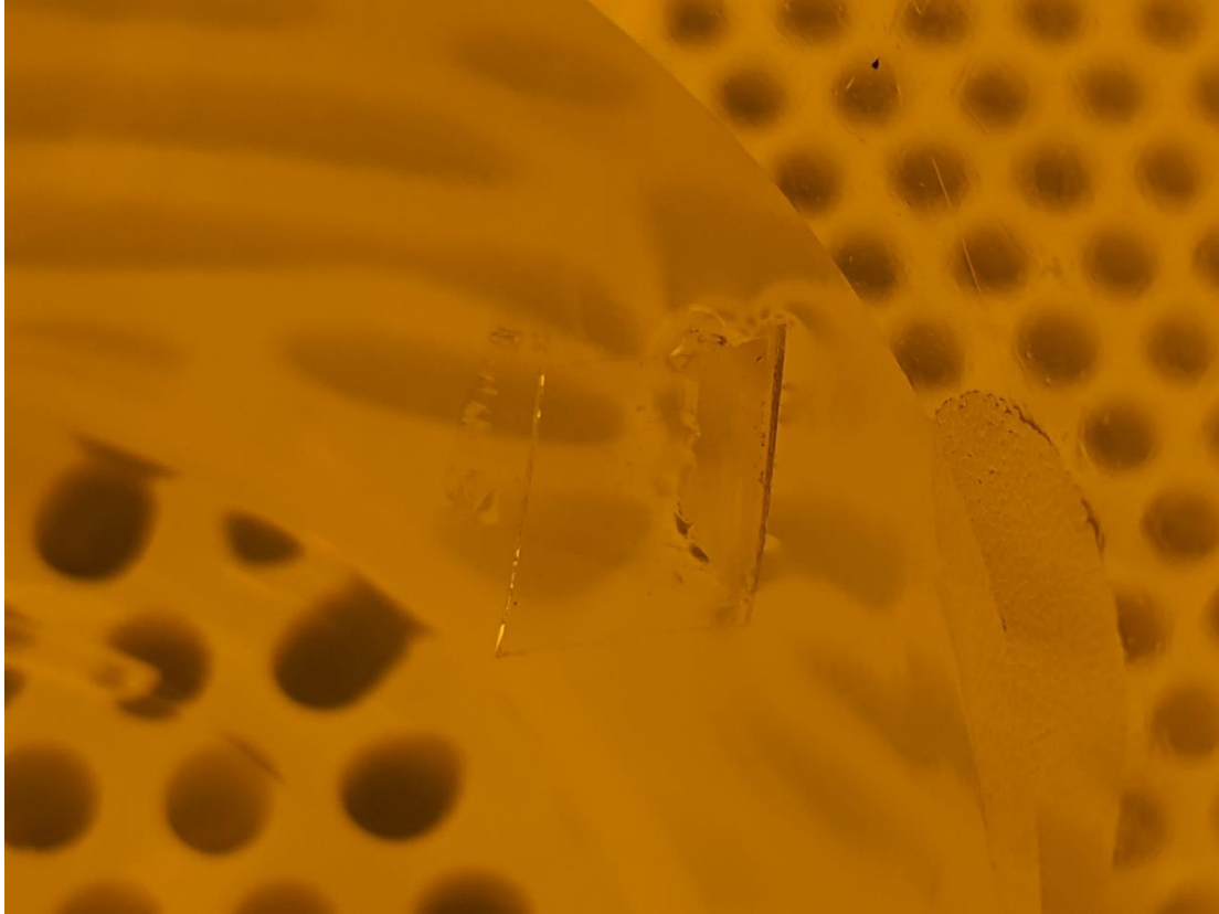
Figure 48. Close up view of the PMMA/CVD 2D material naturally being delaminated from the sapphire substrate prior to the sapphire substrate sinking into the BOE solution.
