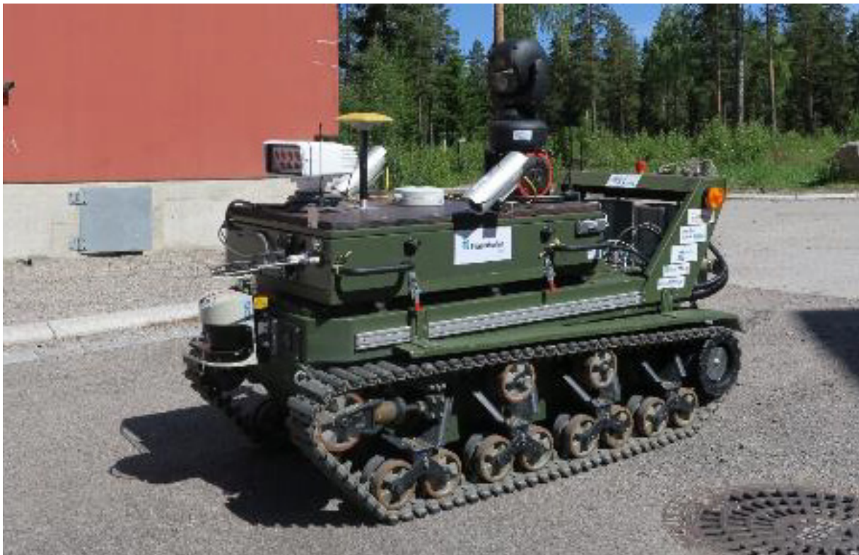
Figure 8-4: Robot Chassis GARM from RUAG and Payload from FKIE.
