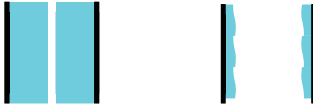
Figure 14: Visual depiction of the rocket motor with port before and after firing. Uneven burning results in difficulty of measuring final grain port diameter.
