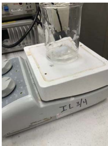
Figure 8: Image of polyethylene melting into paraffin while being stirred magnetically.
