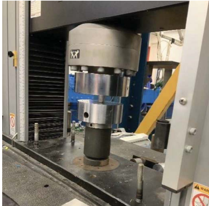
Figure 11: Image of the load frame used for testing with a sample in the test cell.
