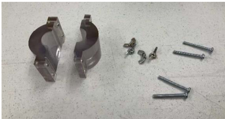
Figure 7: An image of the split mold created for sample synthesis.
