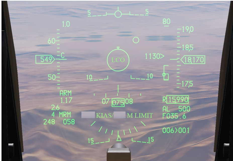
Figure 17: Mockup LCO Recovery display in the HUD, created using a screenshot of the HUD from DCS. A flashing “LCO” appears in the middle of the screen, similar to a low fuel warning. The limits are also displayed in the lower middle of the screen for easy reference.
