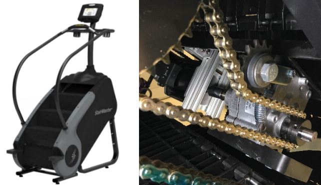
Figure 9: Stair Descent Machine. We have replaced the resistive alternator with a powered motor for reverse direction operation.
