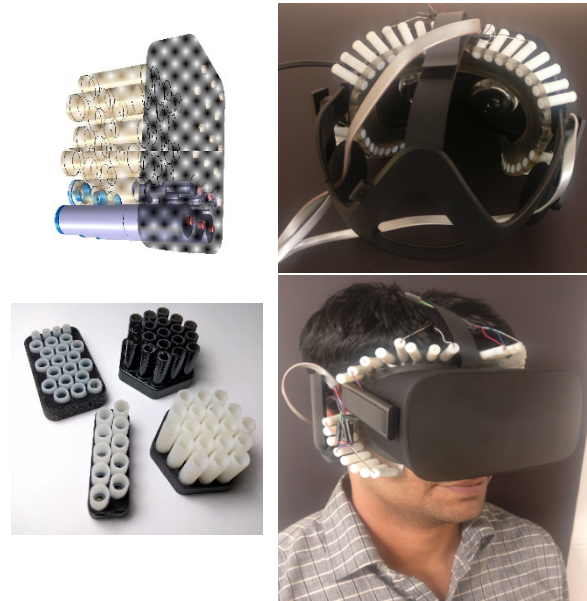
Figure 2. High Density Cam- design for arrays (left) and integrated with a virtual reality headset (right.)
