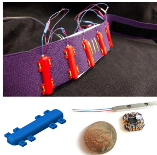
Figure 4. An array of powerful piezoelectric vibrotactors in custom housings along a thigh band for foot placement cues.
