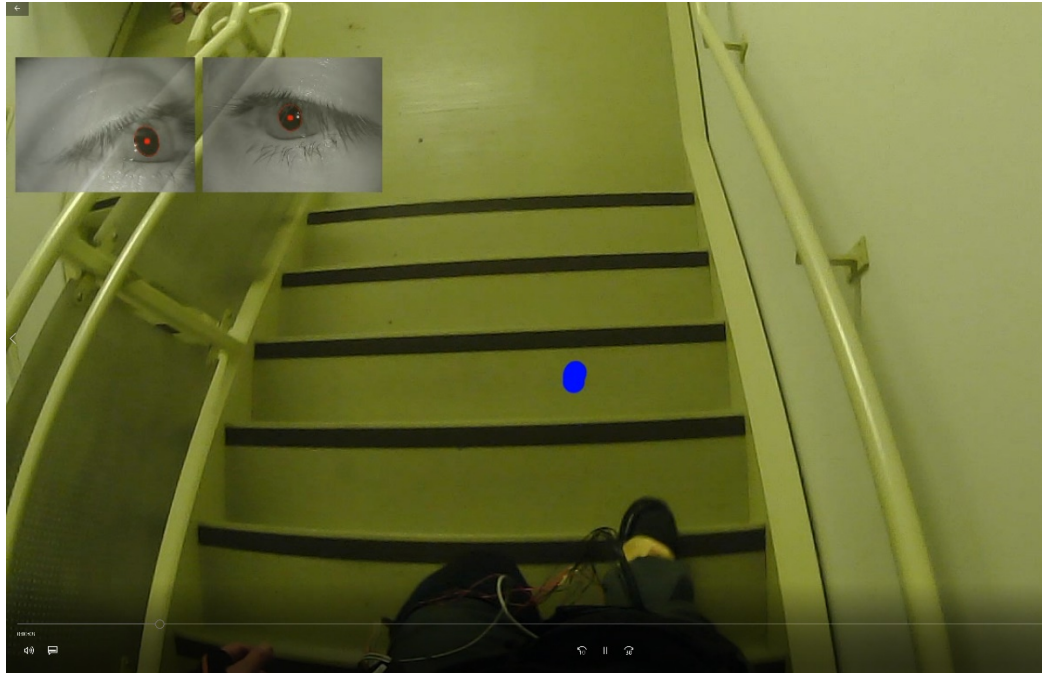
Figure 14: Full stair ambulation test including full body kinematic recordings and eye gaze tracking for quantification of performance changes under stimulation.
