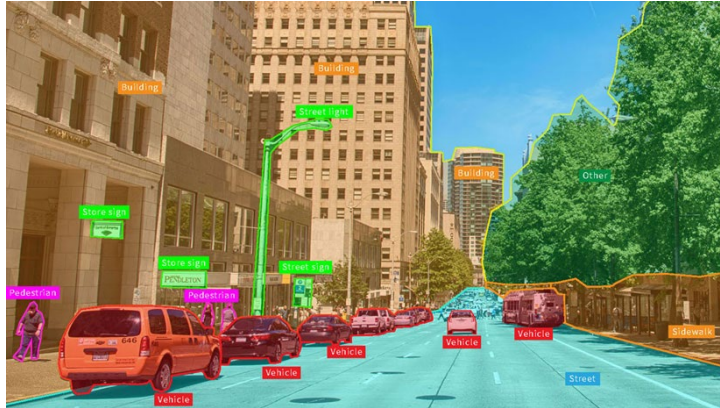
Fig. 1 Example pixel-wise annotation of an urban environment. A human annotator must draw the boundaries between every object in the scene and then assign a semantic label. Each color in this image represents a different semantic class.
