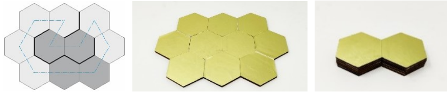
Fig. 2 The Hamptonian cycle (blue lines) for a flat surface made form hexagons and its folding into two compact stacks. Thick black edges of hexagons are slits.
