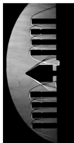
Figure 12: Schlieren photograph of MAP at Mach 5.
