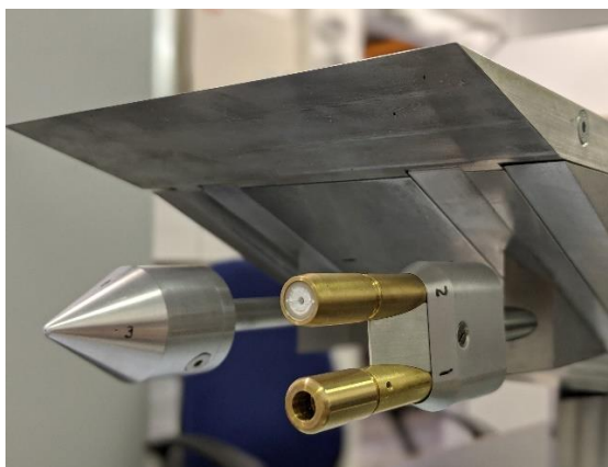
Figure 9: Twin-probe (on the right), with one probe un-instrumented and Model Alignment Probe (on the left) installed on a DSTL-sponsored flat-plate model.
