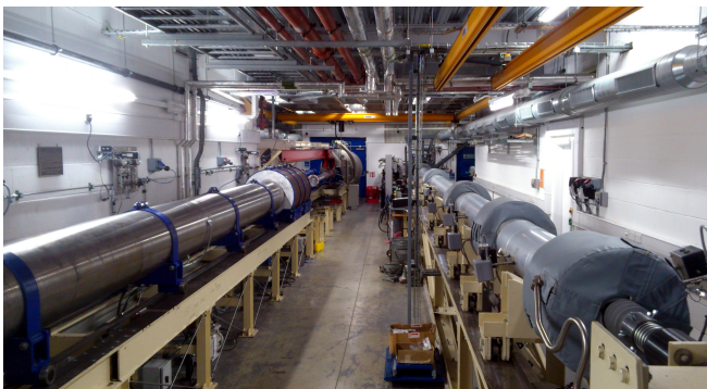
Fig. 8. Hypersonics Laboratory at the Oxford Thermofluids Institute. The T6 Stalker Tunnel is on the left and the High Density Tunnel is on the right.
