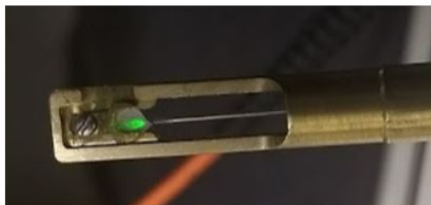
Fig 2: (top) TEM holder with an optical feedthrough and 3-axis micrometer stage; (bottom) top view of the tip of the holder showing laser beams of various wavelengths incident on the substrate.
