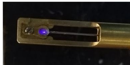
Fig 2: (top) TEM holder with an optical feedthrough and 3-axis micrometer stage; (bottom) top view of the tip of the holder showing laser beams of various wavelengths incident on the substrate.
