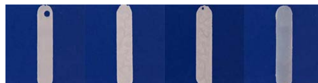
Figure 2. Images of SBE films for different curing temperatures and processing methods: 70, 80, and 90 °C and UV-cured (left to right).
