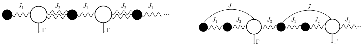
Figure 2 Left (right) panel: dissipative dimer (trimer) chain. Black dots are qubits and open dots are lossy cavities. The couplings J_i are various qubit-cavity interactions.
