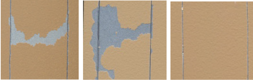
Fig. 14 SurTec 650-sealed IVD Al on AA 2024-T3 (L), Ti 4AL 6V (C), and 4130 steel (R)
