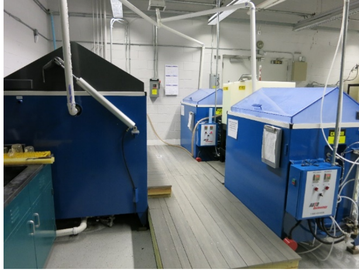
Fig. 1 Neutral salt-fog corrosion chambers used for testing
