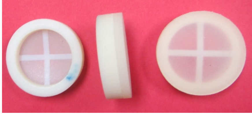
Fig. 8—Halves of cylindrical inclusions designed with the beam element and outer ring fabricated from DigitalABS and a top layer fabricated from TangoPlus
