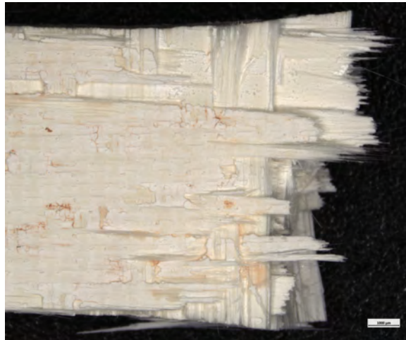
Figure 62. Optical micrograph of a N720/AM specimen fracture surface tested in tension-tension fatigue at 1200°C in air. \sigma_{\max} = 130 MPa, N_f > 100,000
