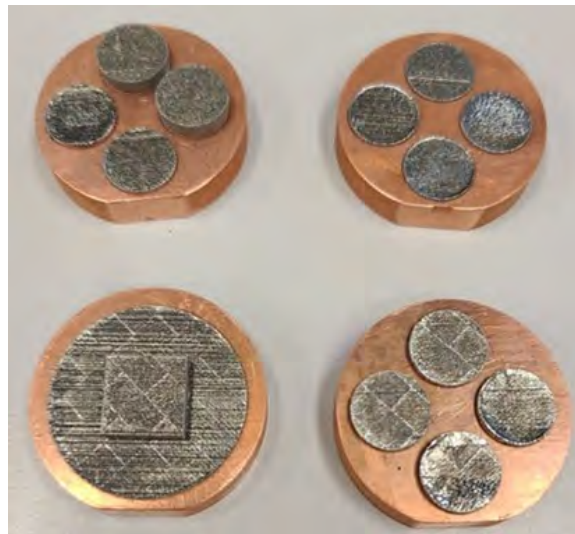
Figure 7. Four Cu individual print surface pucks with various WReHfC prints
