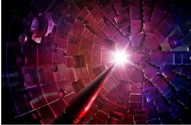
Figure 11. Target Chamber of the National Ignition Facility at LLNL with 192 Laser Beams Converging on a Target in the Containment Sphere
