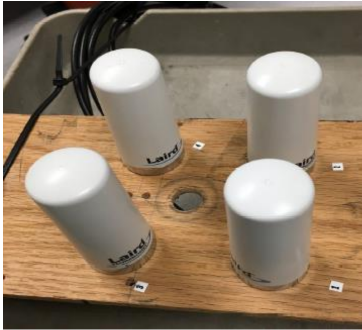
Figure B1: Laird Technologies LTE Antennas Prior to Installation on the C-12J
