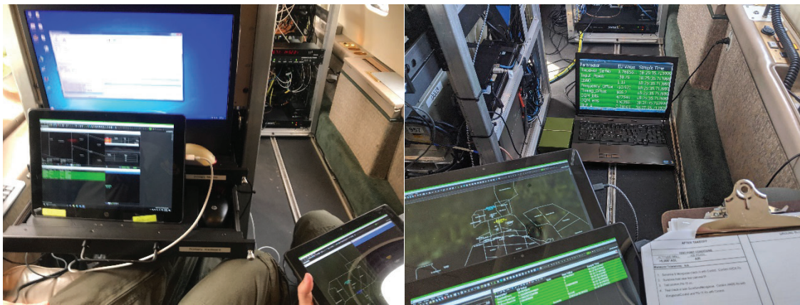
Figure 4 – Terminator Pod System Left and Right Operator Stations in the Sabreliner. Tablets Running NetView are Shown (Left and Right)
