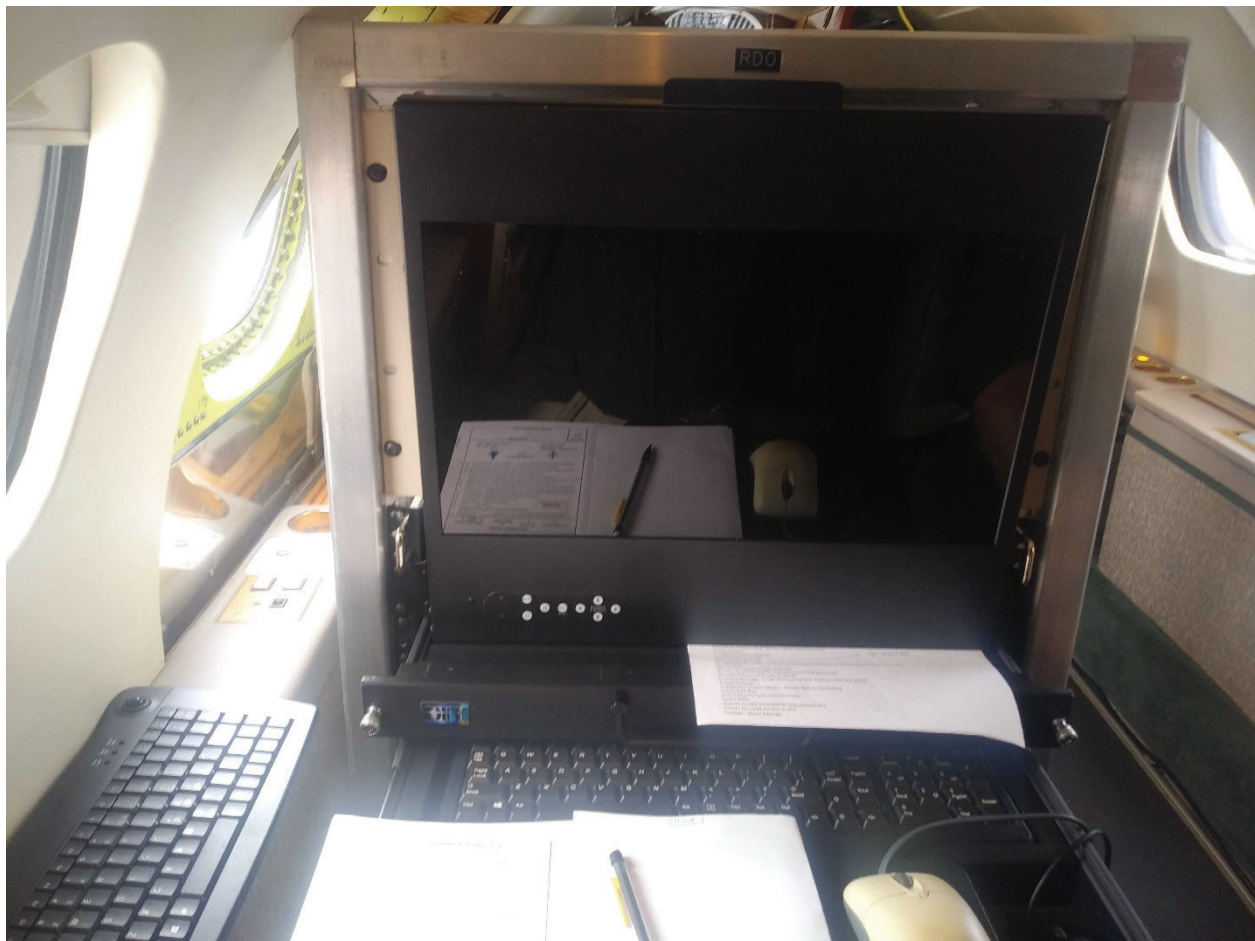
Figure 14 – Left-Hand Operator Station. Two Keyboards (Center and Left), Two Mice (Bottom Right) and the PC Screen (Center) are Shown. Tablets Not Shown
