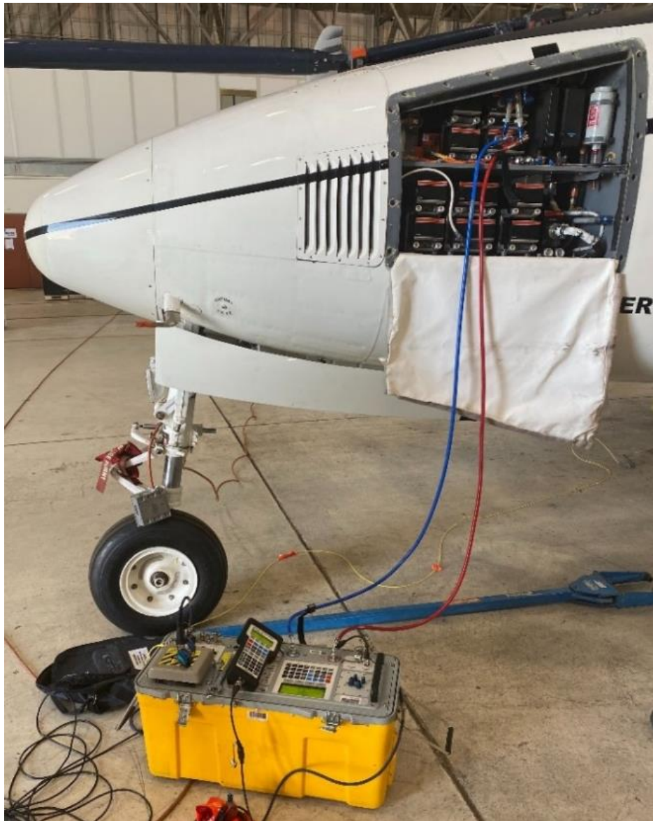
Figure A2. Druck™ ADTS 405 Connected to ADC 1
