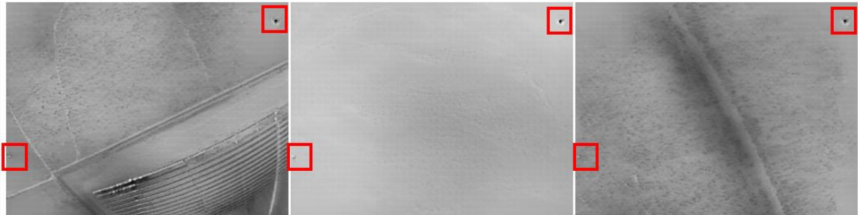
Figure 13 Non-Physical Artifacts Consistently Generated by Front End Neural Network
