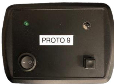
Figure 8. Psychomotor Vigilance Test box. Participants performed a three-minute reaction time test in which they pressed the right button with the right index finger in response to the blue light turning on. A green light signaled the end of the test.
