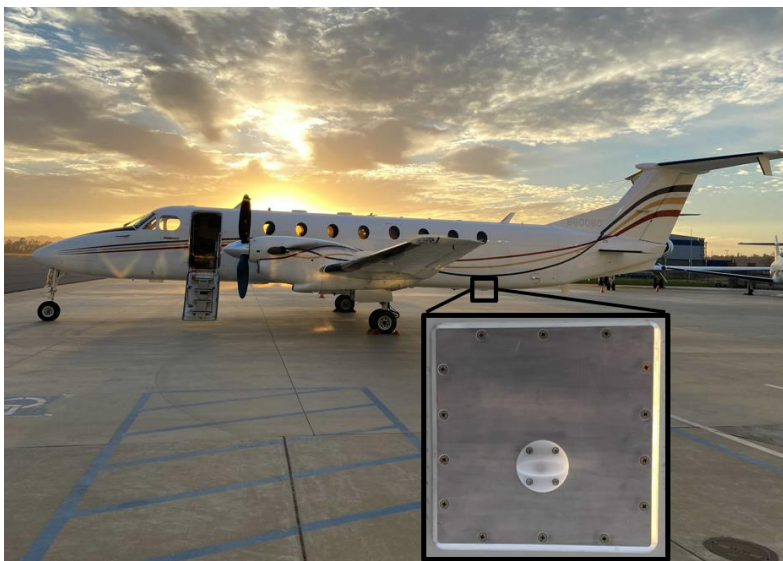
Figure I-1: C-12J with Monopole Antenna Location
