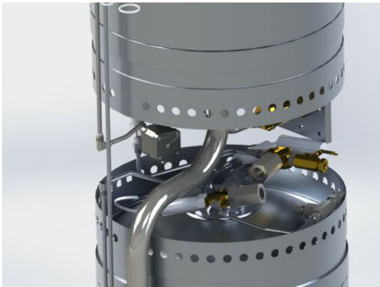
Intertank Bay Plumbing - Solidworks
