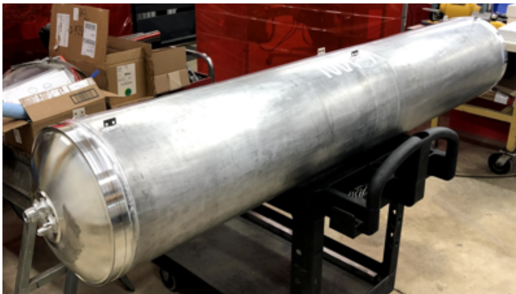
Figure: LOX Flight Tank immediately after Full Assembly Welding
