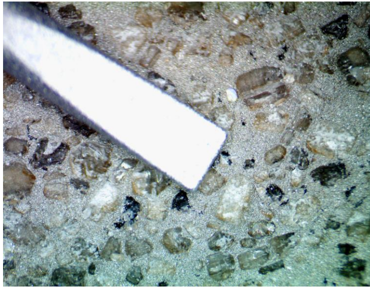
Figure 19: Inert propellant with 1000 \mu\text{m} wide screwdriver blade. Flat punch indenter used for dynamic micro-indentation measures 53.1 \mu\text{m} dia.
