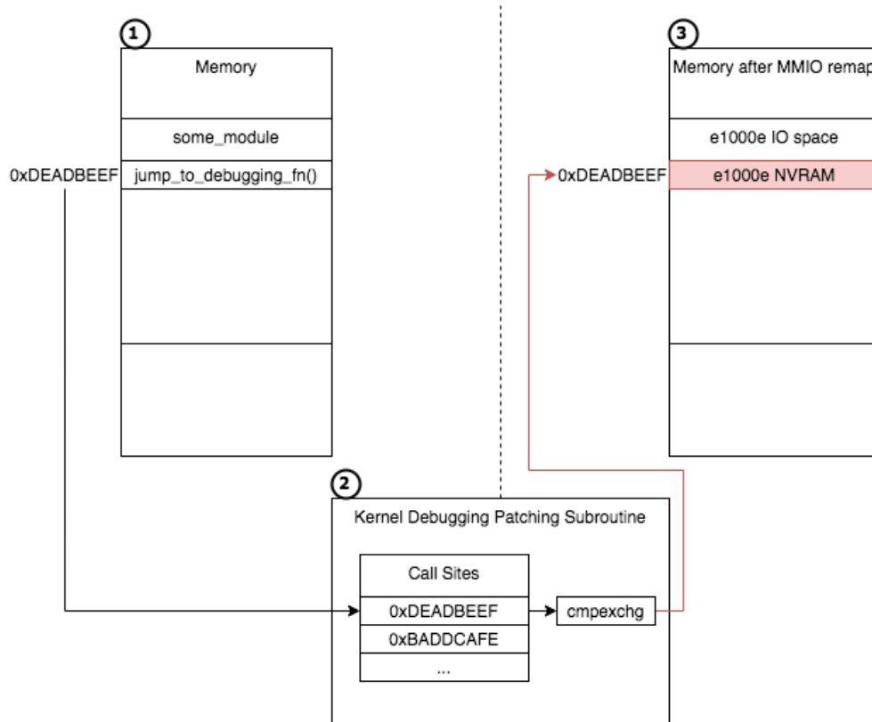
Figure 2-4: The e1000e bug: In 1, the memory is loaded with an arbitrary module. To enable debugging, the compiler adds a function jump at the beginning of the module. In 2, the kernel has a runtime patching subroutine which notes all debugging function call sites and patch the debug function jump if debugging is not enabled. 3 shows a view of the memory after the module is freed and the e1000e is mapped to where the module used to be. Unfortunately, the cmpexchg instruction executes since it still believes 0xdeadbeef is the callsite and accidentally writes to the e1000e NVRAM space, destroying the device.
