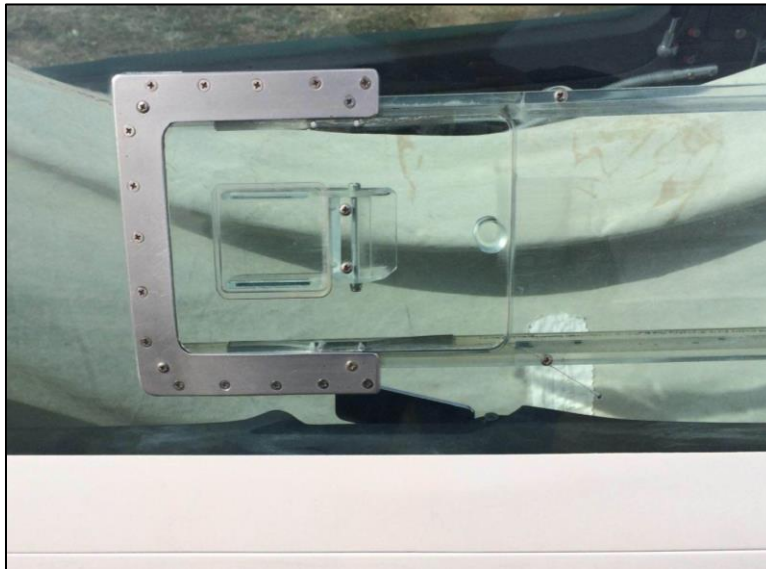
Figure B-8 DG-1000S N801DG Window Reinforcement Bracket.
