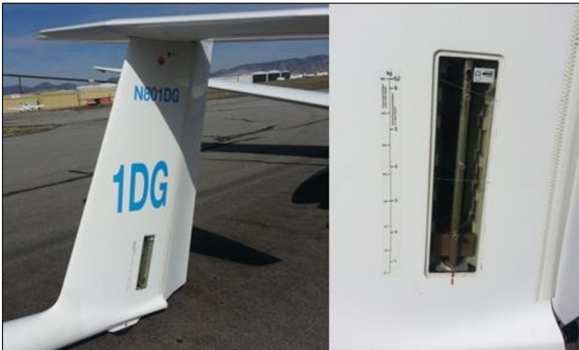
Figure B-4: DG-1000S N801DG Tail Ballast Boxes.
