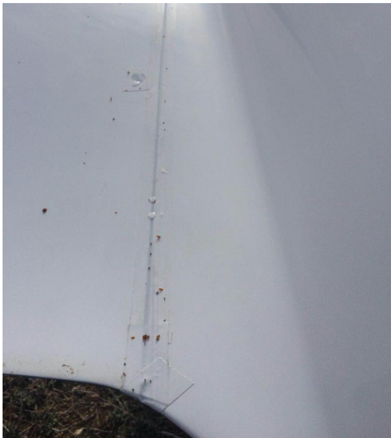
Figure B-12 DG-1000S N801DG Wing Attach Point Taped Seam
