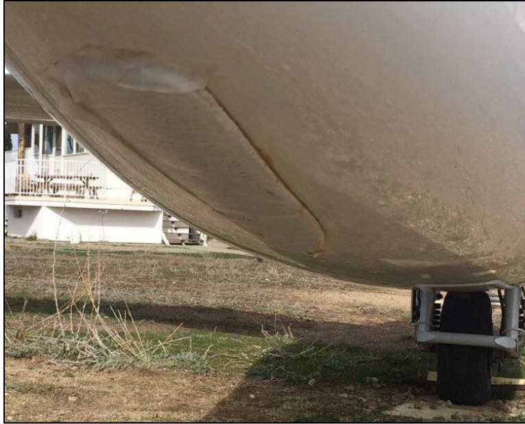
Figure B-7: DG-1000S N801DG Skid Plate.
