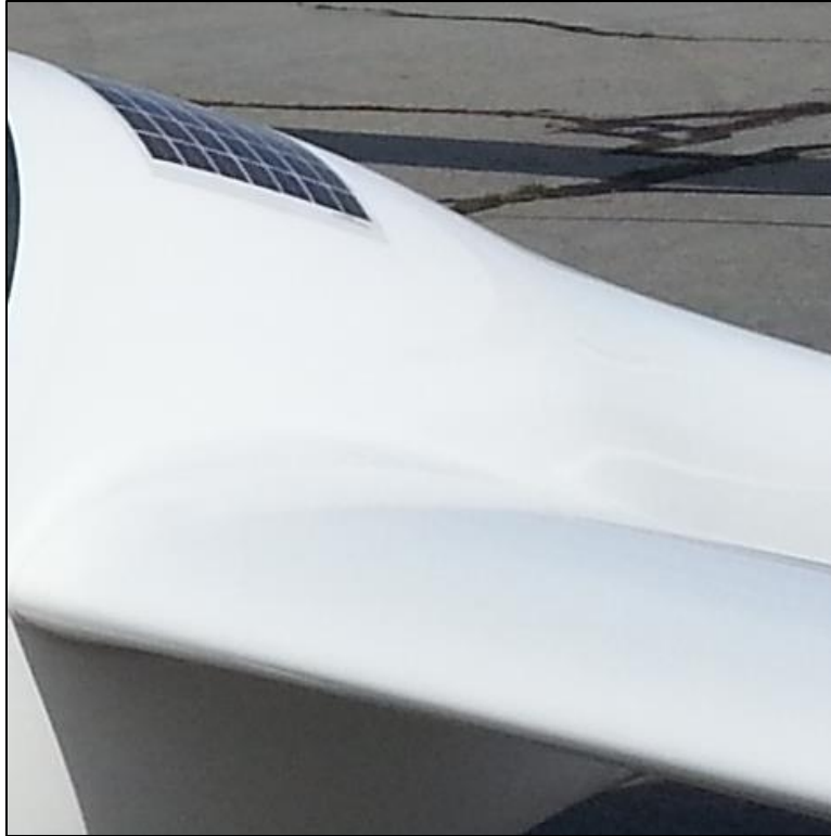
Figure B-9 DG-1000S N801DG Solar Panels.
