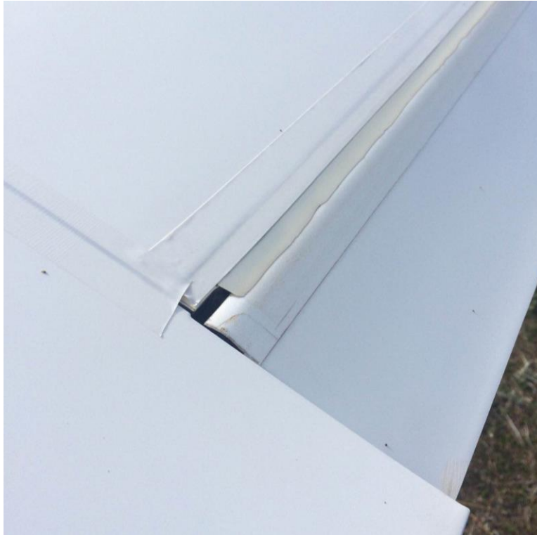
Figure B-11 DG-1000S N801DG Aileron Taped Seam.
