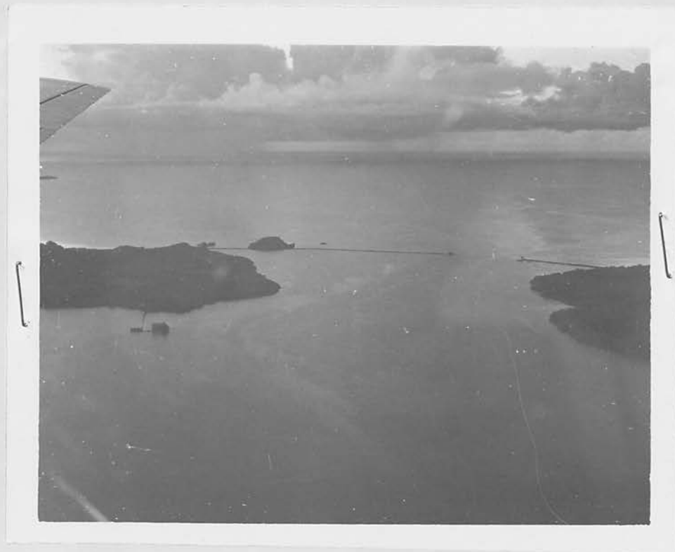
Illustration 4: Aerial view looking west of ferry channel between Koror on the left and Babelthuap on right. Long moles have been built on coral shelving; ship channel is approximately 300 yards wide and 120 feet deep.
