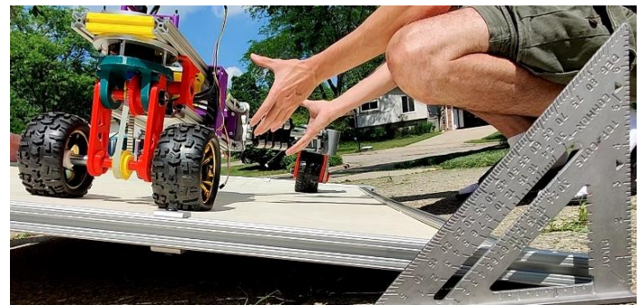
Figure 15: Experimental Tilt Test (Prior to Leg Reinforcement)
