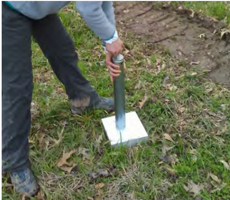
FIGURE 3.8: Impact source: standard proctor hammer and aluminum plate
