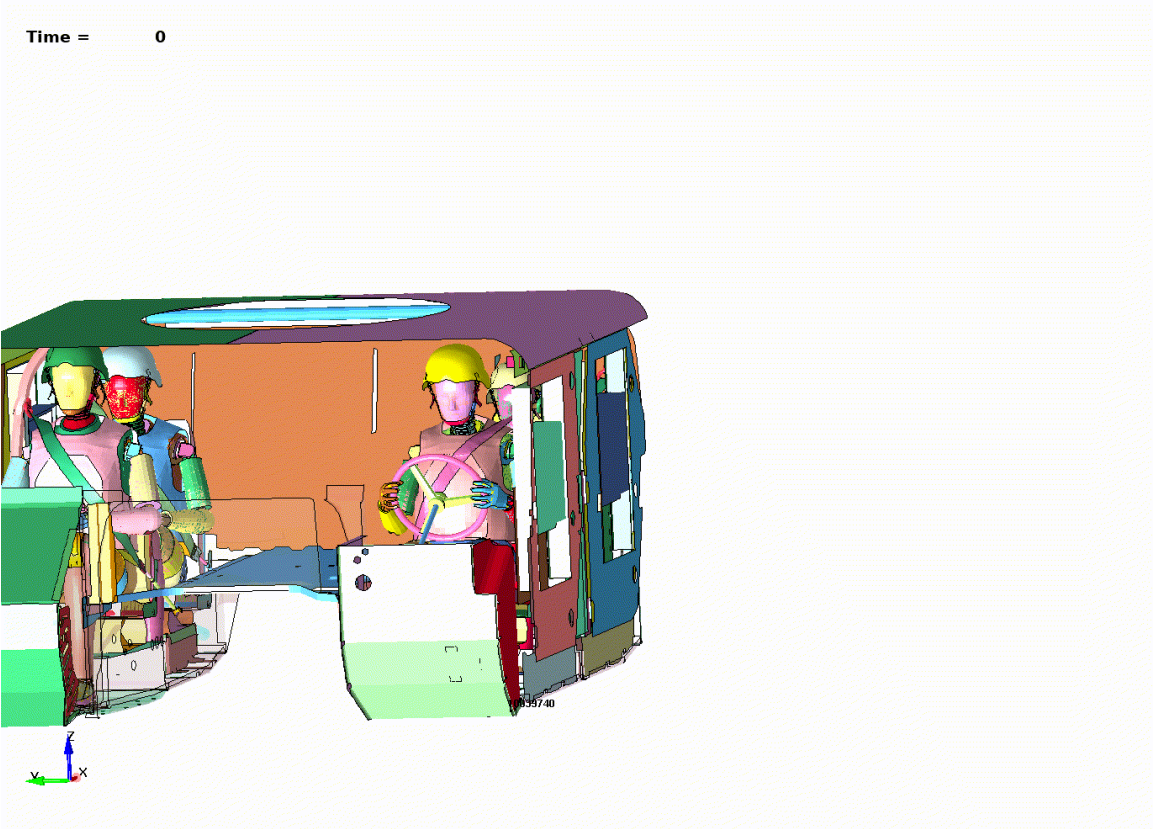
ROMM Model with occupants and seatbelt restraints system
