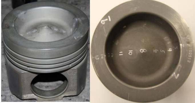
Example of new piston, pre-test (note Mn phosphate coating)
