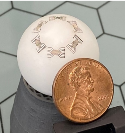
Practice circuits on 1" dia. Delrin ball.
