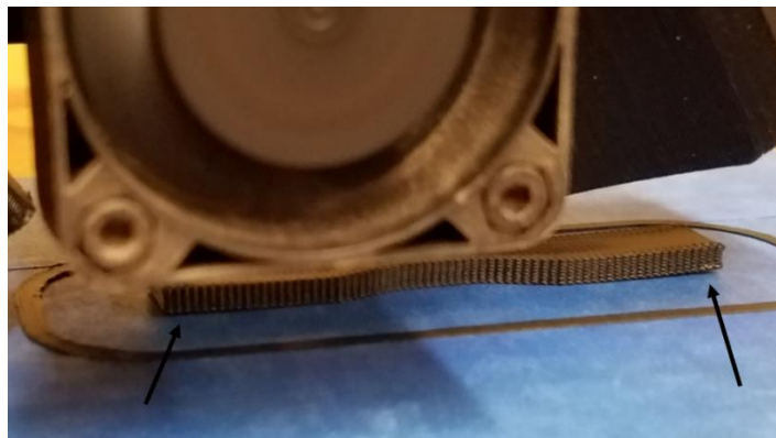
Figure 13. Small scale print evidence of warping as print pulls off the bed during print
