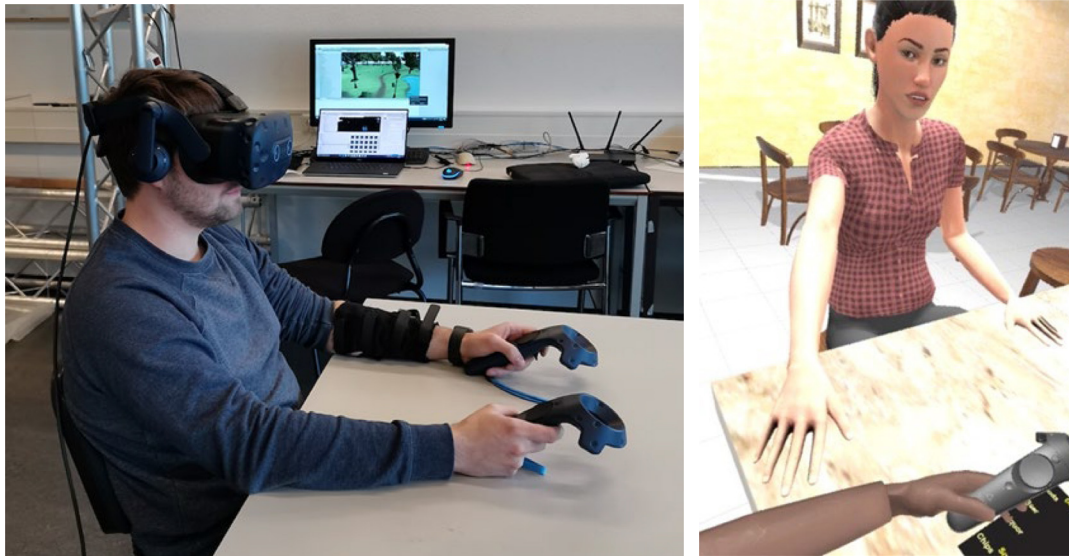
Figure 1. The virtual reality setup. Left: A participant wearing the vibrotactile sleeve on the left forearm, holding the movement trackers and wearing the VR head setup. Right: The virtual environment (bar) with the VA that were used in the study. The VA reaching towards the user's forearm just before the touch.
