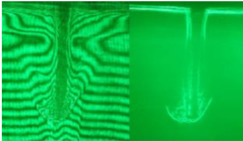
Fig. 16. 0.5mm rod suspended along direction of plasma flow in jet from radial foil. Left: Interferometry image. Right: shadowgraphy image.
