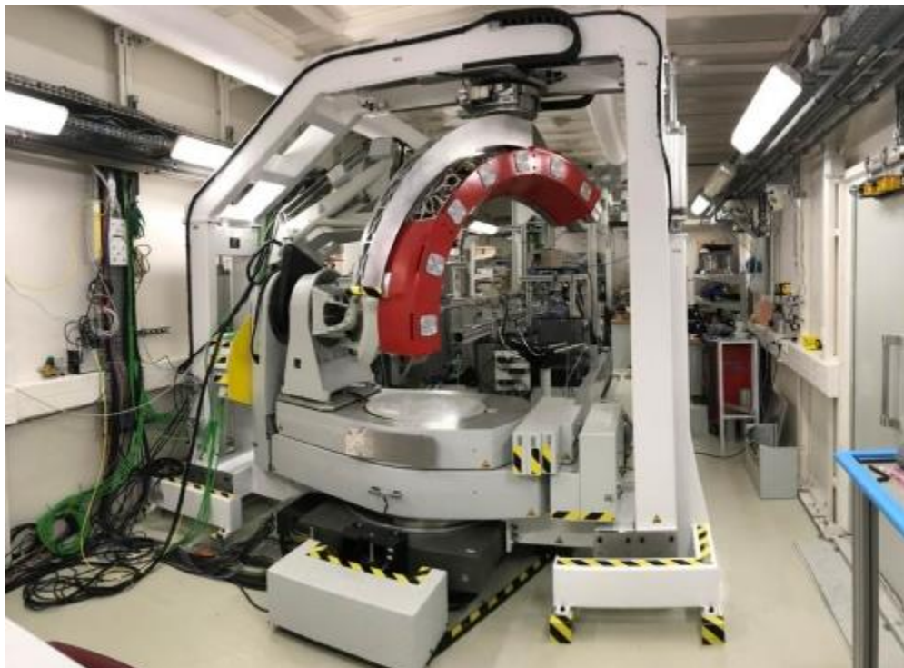
Figure 2. CirPAD detector of Diffabs beamline in Soleil Synchrotron.
