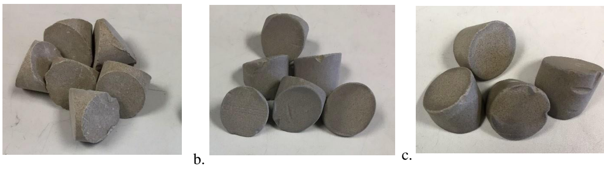
Figure 14. Synthetic Rocks. a. Original; b. Test Set 1 With Layer of Dust/Dirt (945 min or 15.75 h of abrasion time); c. Test Set 1 Washed after Testing (945 min or 15.75 h of abrasion time)
