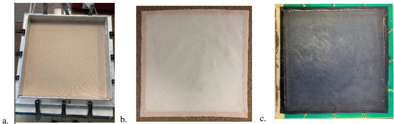
Figure 6. Preliminary Testing a. Fabric Mounted in Frame; b. Modacrylic Blend Abraded 60 min, Frame Removed; c. FR Cotton 60 min, Frame Removed
