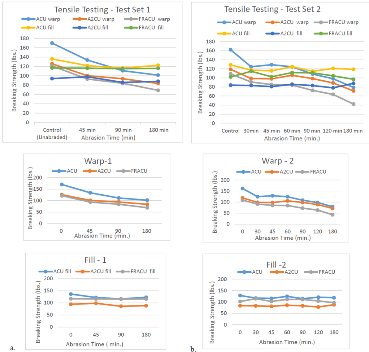
Figure 12. Tensile Test Results. a. Test Set 1; b. Test Set 2
