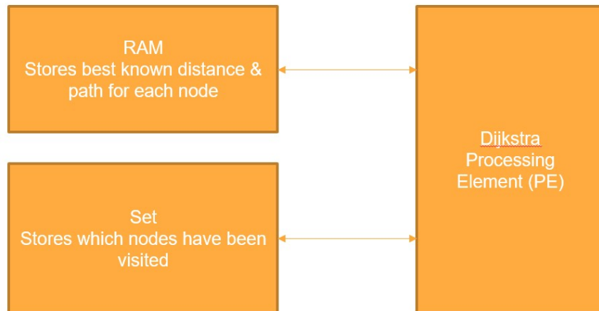
Figure 10: A High Level Drawing of the Dijkstra Algorithm Implemented in VHDL The RAM and Set have been designed so that many copies of the Processing Element (PE) can run in parallel.
