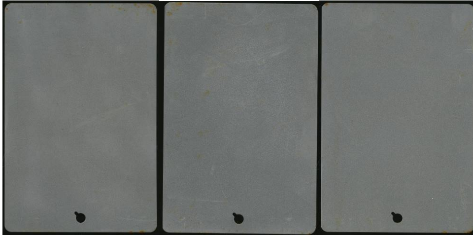
Fig. 14 Humidity test results on Type Z panels sealed with SurTec 555
