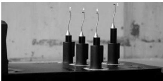
(b) probes used to measure airwake velocities
