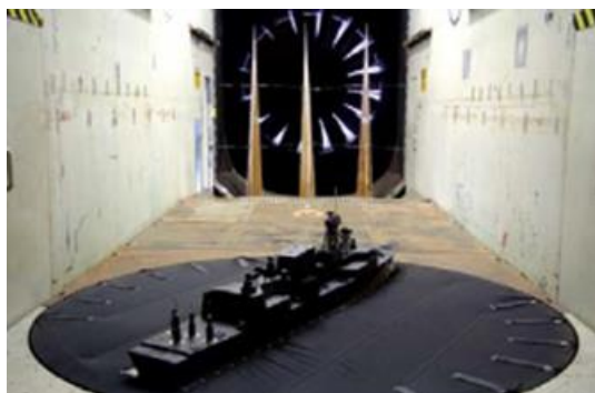
(a) wind tunnel setup
